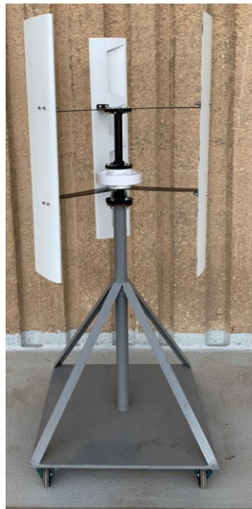
Figure 4.5 Wind Turbine Assembly
