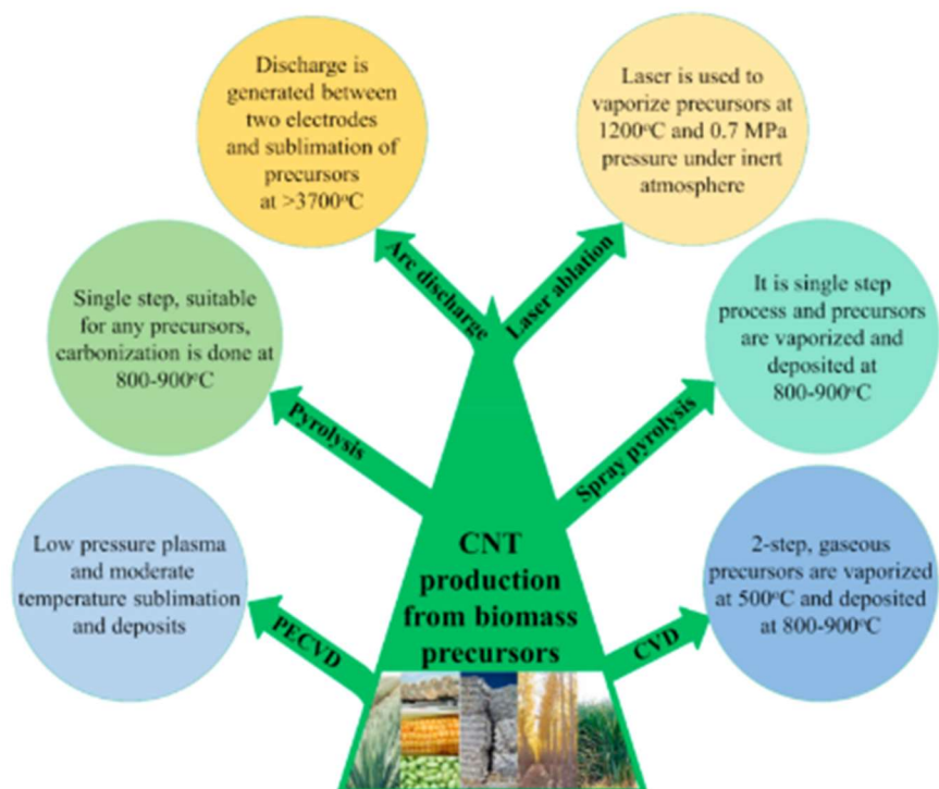
Figure 2.12. CNT production from biomass based on different synthesis procedures (Hoang, Nižetić, et al., 2022).
