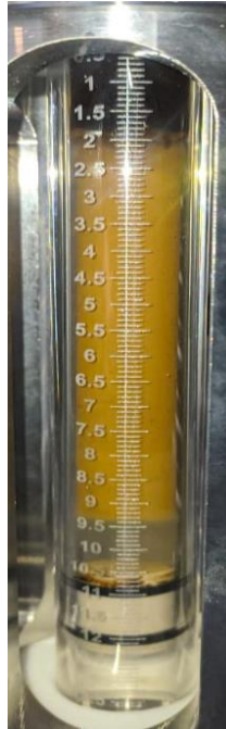
Figure 68: 17283 ppm GOR 180, P = 3000 psi, T = 90°C.
