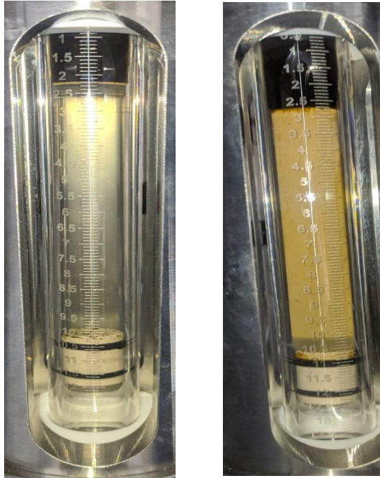
Figure 66: 11522 and 12962 ppm GOR 180, P = 3000 psi, T = 90°C.
