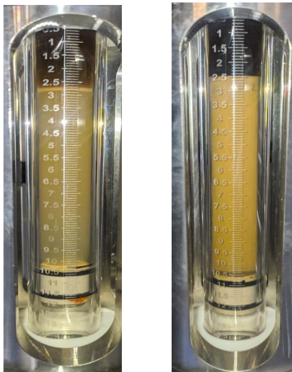
Figure 67: 14403 and 15843 ppm GOR 180, P = 3000 psi, T = 90°C.
