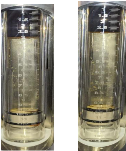
Figure 73: 14403 and 15843 ppm GOR 380, P = 3000 psi, T = 90°C.
