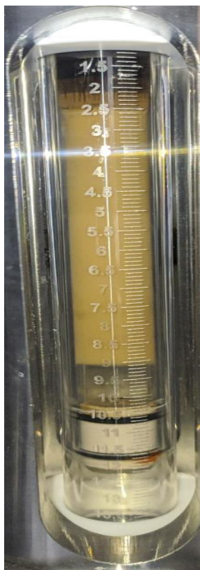
Figure 58: 14403 ppm GOR 280, P = 3000 psi, T = 90°C.
