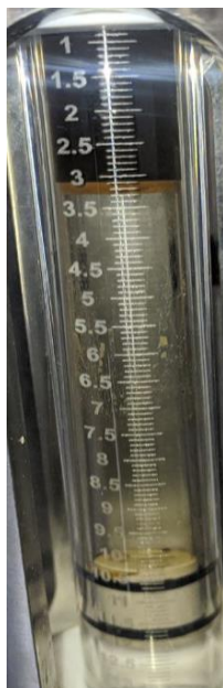
Figure 74: 17283 ppm GOR 380, P = 3000 psi, T = 90°C.
