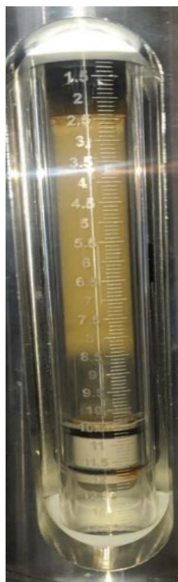
Figure 61: 14403 ppm GOR 280, P = 3500 psi, T = 90°C.
