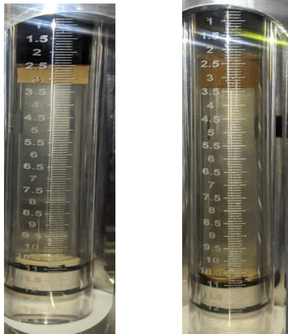
Figure 65: 15843 and 17283 ppm GOR 180, P = 2500 psi, T = 90°C.
