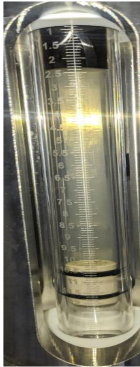
Figure 63: 11522 ppm GOR 180, P = 2500 psi, T = 90°C.
