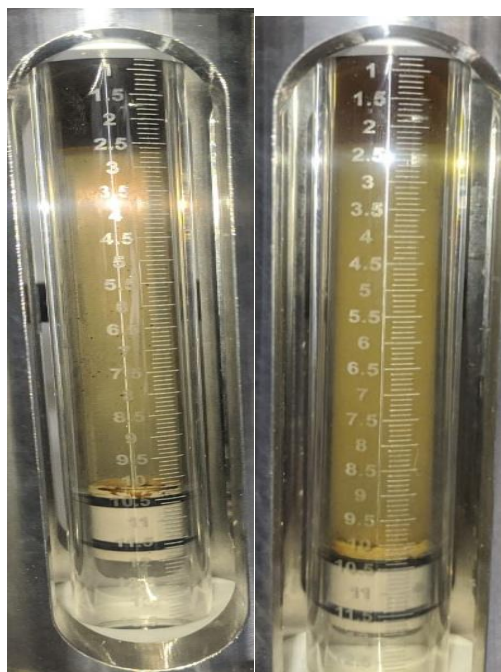
Figure 56: 15843 and 17283 ppm, GOR 280, P = 2500 psi, T = 90°C.
