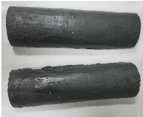
Figure 14. The sample after covering by epoxy
