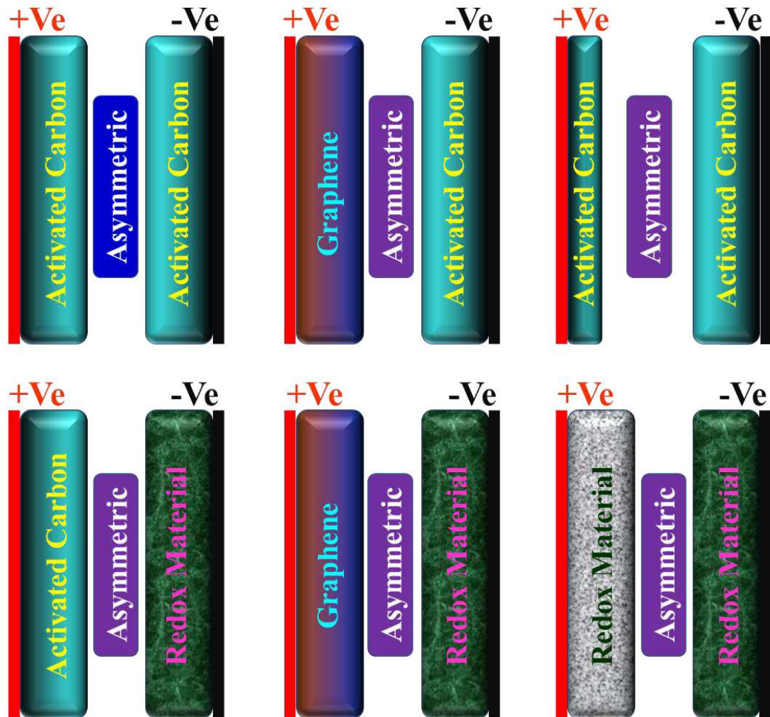
Figure 1.4. Schematics for the symmetric and asymmetric configuration of supercapacitors.
