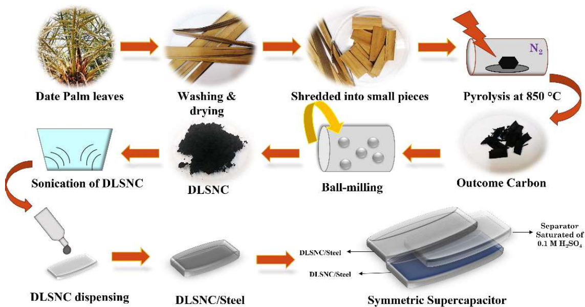
Figure 3.1. Schematic representation for the DLSNC synthesis and the DLSNC/Steel based symmetric supercapacitor device fabrication.
