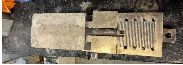
Figure 21: Typical assembly of beam-bend test specimen with the apparatus
