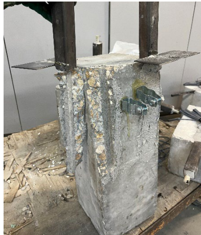
Figure 45: Failure pattern of DA-C (DA-C: circular CFRP)
