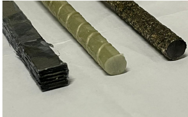
Figure 13: NSM FRP types: CFRP strip (left), GFRP bar (middle), and CFRP square bar (right)
