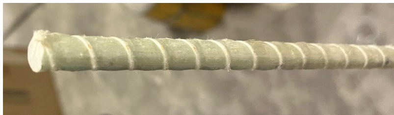
(a) Spirally wound surface GFRP bar with small degree of sand-coating
