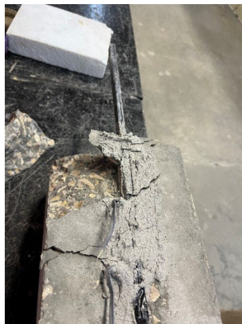
Figure 36: Failure patterns of each specimen (S-G: circular GFRP, S-C: circular CFRP, and S-RC: rectangular CFRP)
