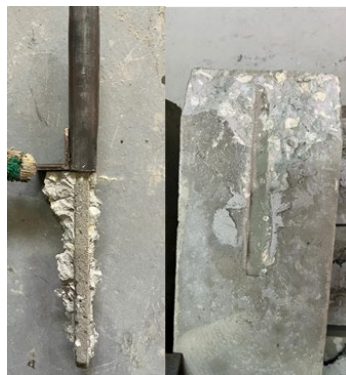
Figure 10: Direct pull-out single-shear NSM FRP-concrete bond test: (a) Specimen details (b) Test setup (c) Typical debonding failure in low-strength concrete [concrete-adhesive interface with degrees of concrete damage] (d) Typical debonding failure in normal-strength concrete [FRP-adhesive interface with partial substrate damage]
