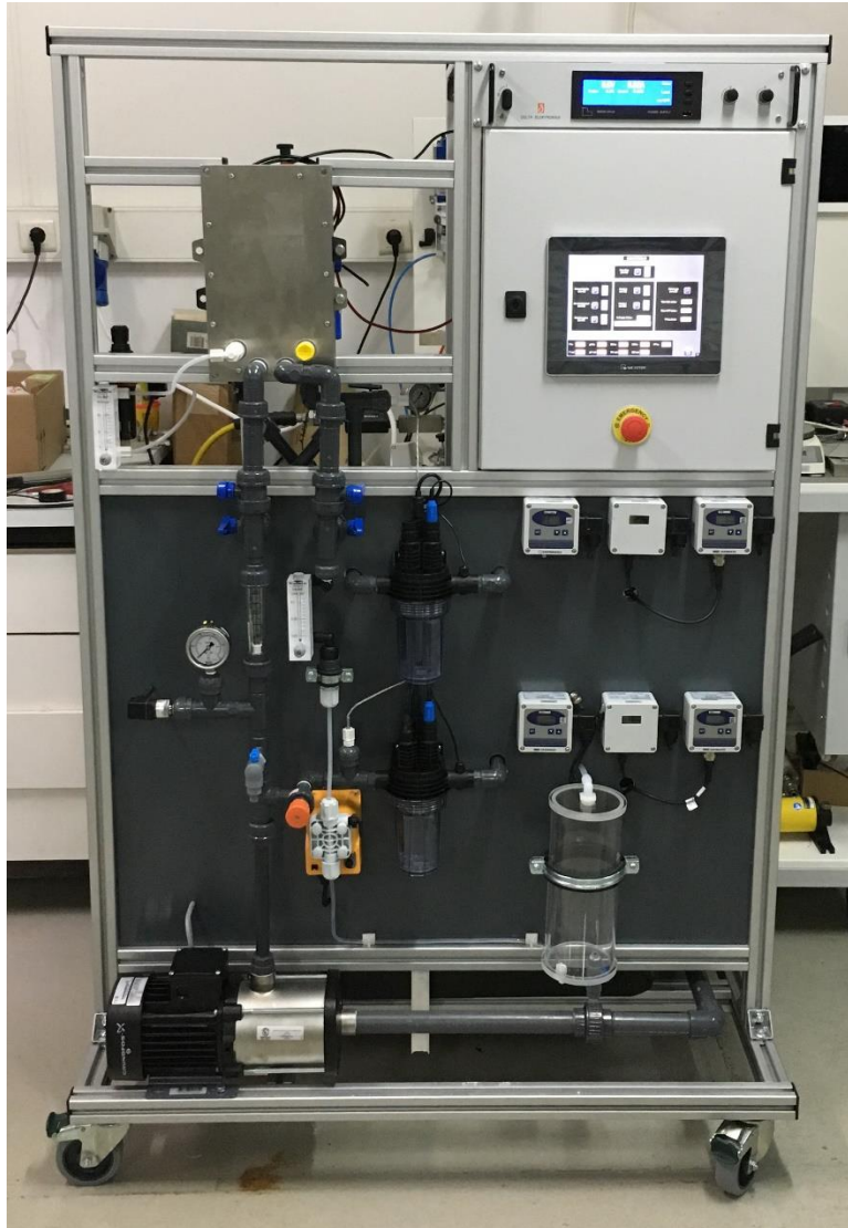
Figure 11: Electrochemical Treatment System (ETS) pilot plant
