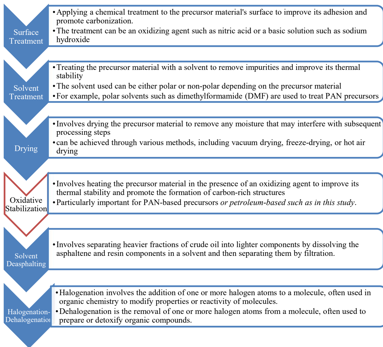
Figure 6 Typical pre-treatment methods used in CF production.
