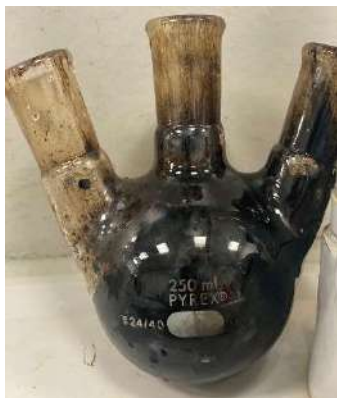
Figure 74 Photograph of heavy black product deposits
