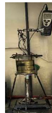
Figure 76 Photograph of manual measuring of softening point using ball-and-ring apparatus
