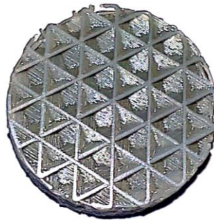
Figure 46 - Showcasing the closed nature of the Pyramidic pattern (no straight pores from end to end)
