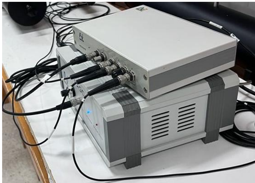
Figure 41 - Top: A multi-channel Data acquisition and single output hardware, Down: 50W power amplifier
