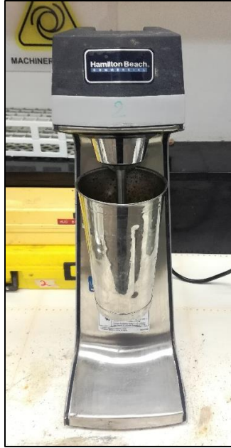
Figure 8 Hamilton drilling fluid mixer
