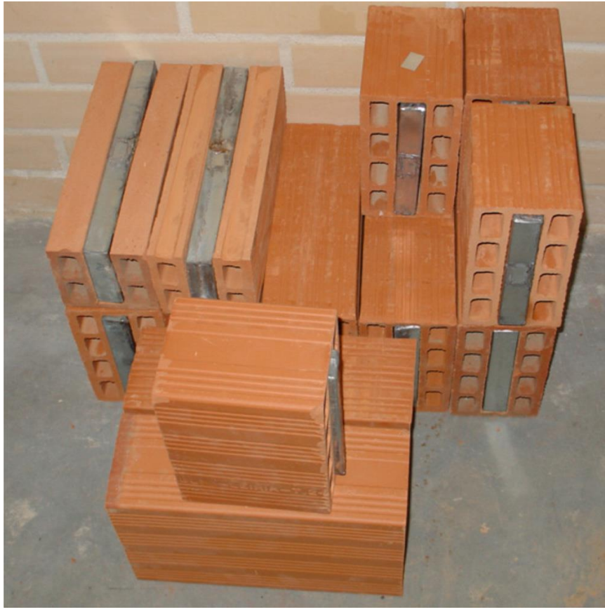
Figure 2.10 Clay bricks containing PCM macro-capsules [51].
