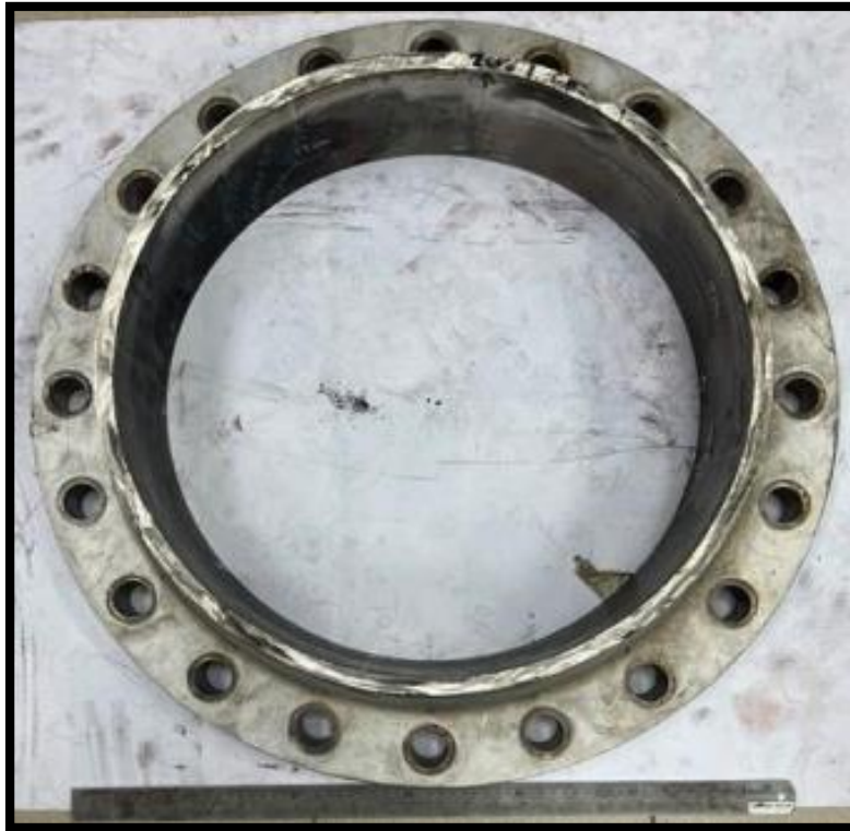
Figure 14: Photo by digital camera showing flange sample as received condition
