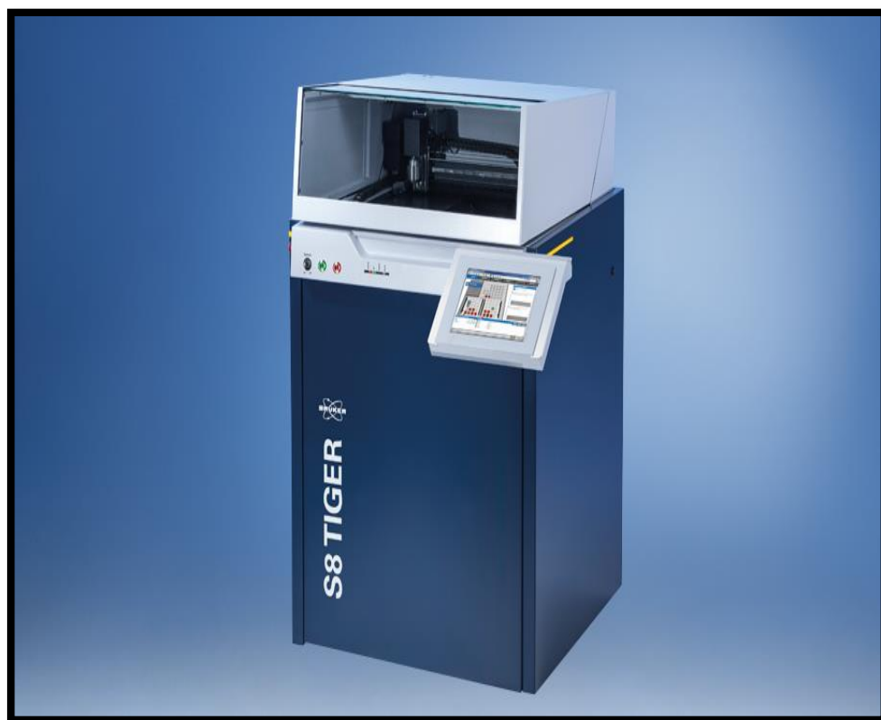
Figure7: X-ray Fluorescence Bruker S8 Tiger
