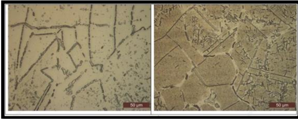
Figure 23: Photos by light microscope of the 1st cracked sample after sensitization test.
