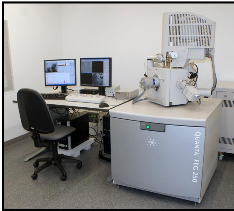
Figure10: Scanning Electron Microscope Analyzer QUANTA FEG 250
