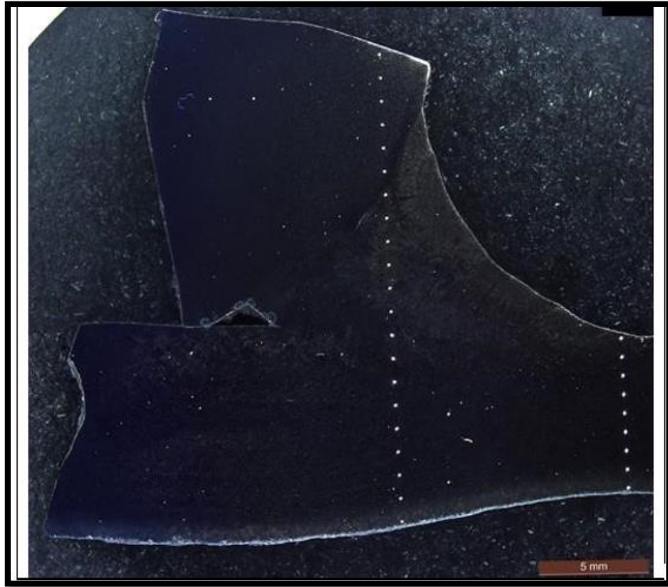
Figure 49: Photo by stereo microscope showing the un cracked sample with indents after hardness test.
