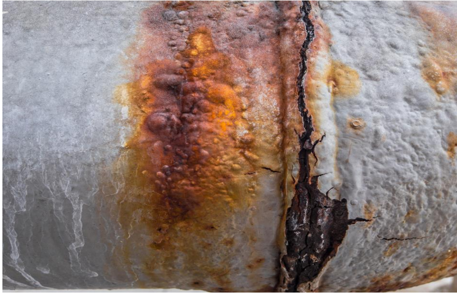
Figure 5: the surface of stainless steel showing clear signs of stress corrosion cracking.
