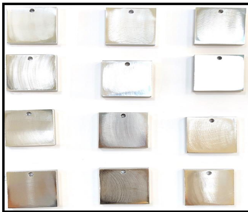
Figure 60: 12 Samples from SS304 L After polishing by Silicon Carbide paper 240 Cw
