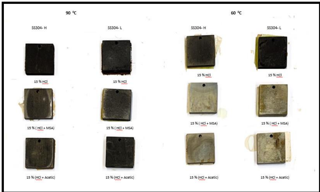
Figure 68: SS304 (H and L) (15%HCl ), (15% MSA &15% HCl ) and (15% Acetic Acid &15% HCl ) at 60 & 90 °C
