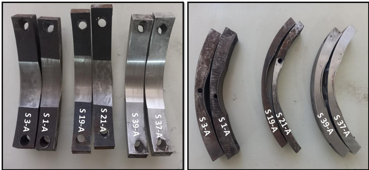
Figure 80. A photograph of the tested P110, L80, and SM2535 casing samples at 115 rpm and two side loads (1400 N and 1000 N) under OBM wet conditions.
