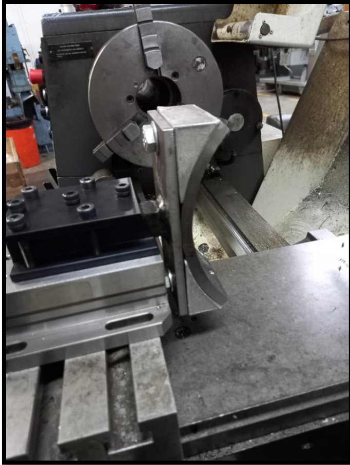
Figure 18. The casing holder mounted on the dynamometer.
