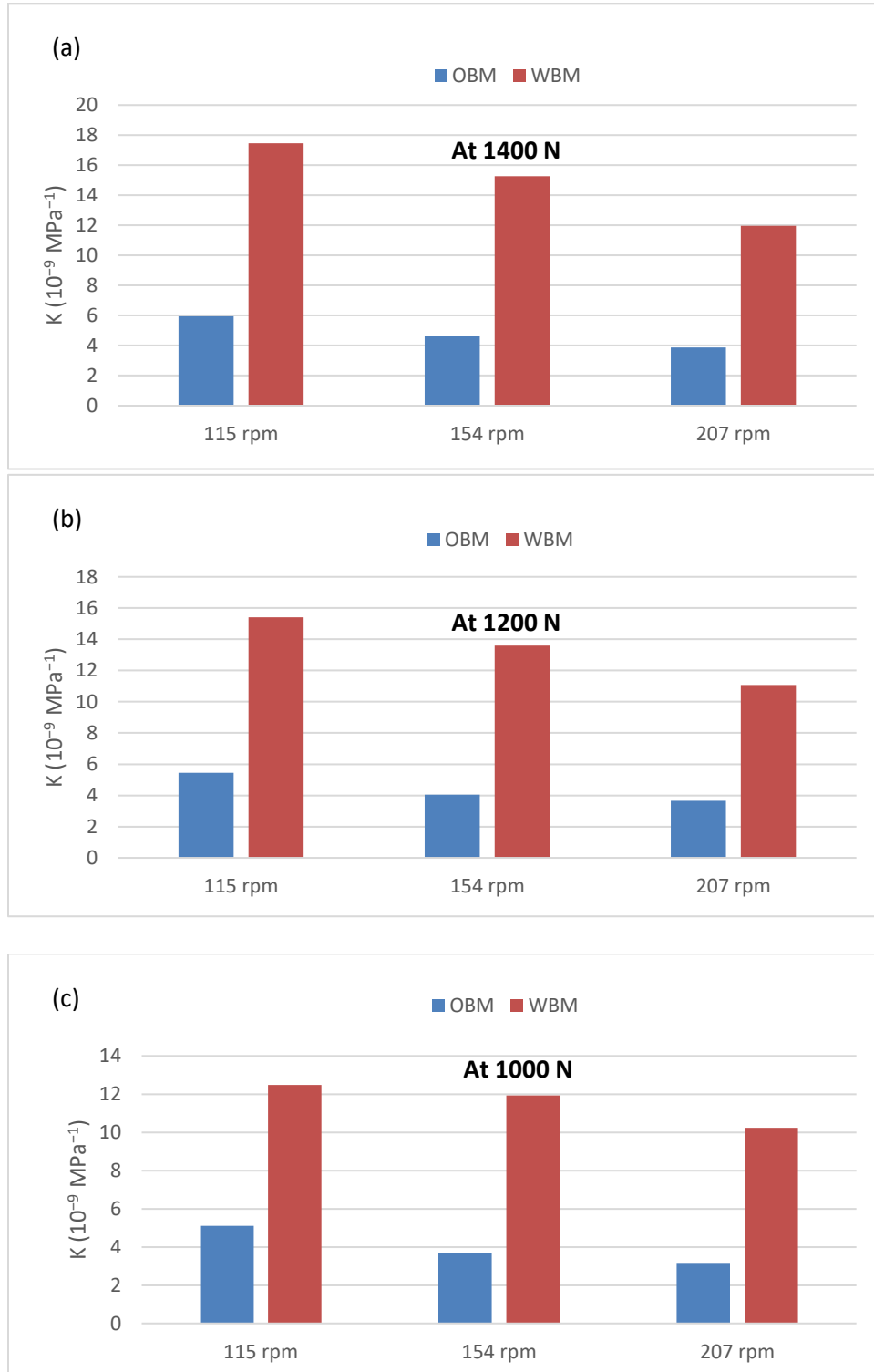
Figure 59. Wear factors of L80 casing sample tested under OBM and WBM at three different speeds (115 rpm, 154 rpm, and 207 rpm) and three different side loads where the side load at a) 1400 N, b) 1200 N, and c) 1000 N.
