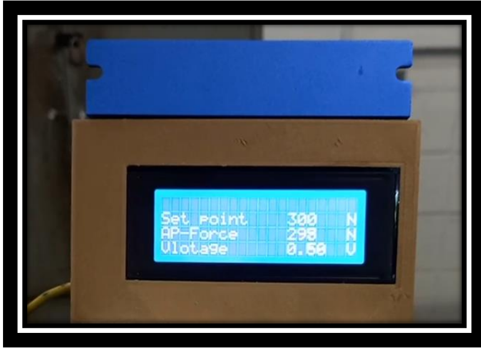
Figure 20. Controlling and monitoring system box.
