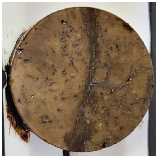
Figure 62 The crack across the Guelph Dolomite sample.
