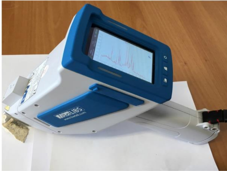
Figure 3 A portable hand-held LIBS device. Reprinted from [6].
