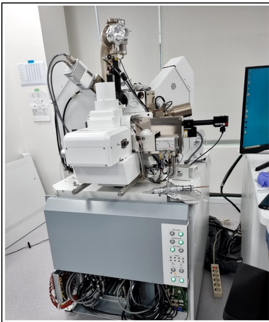
Figure 10 Electron Probe Micro-Analyser, JEOL JXA-8600 SX.
