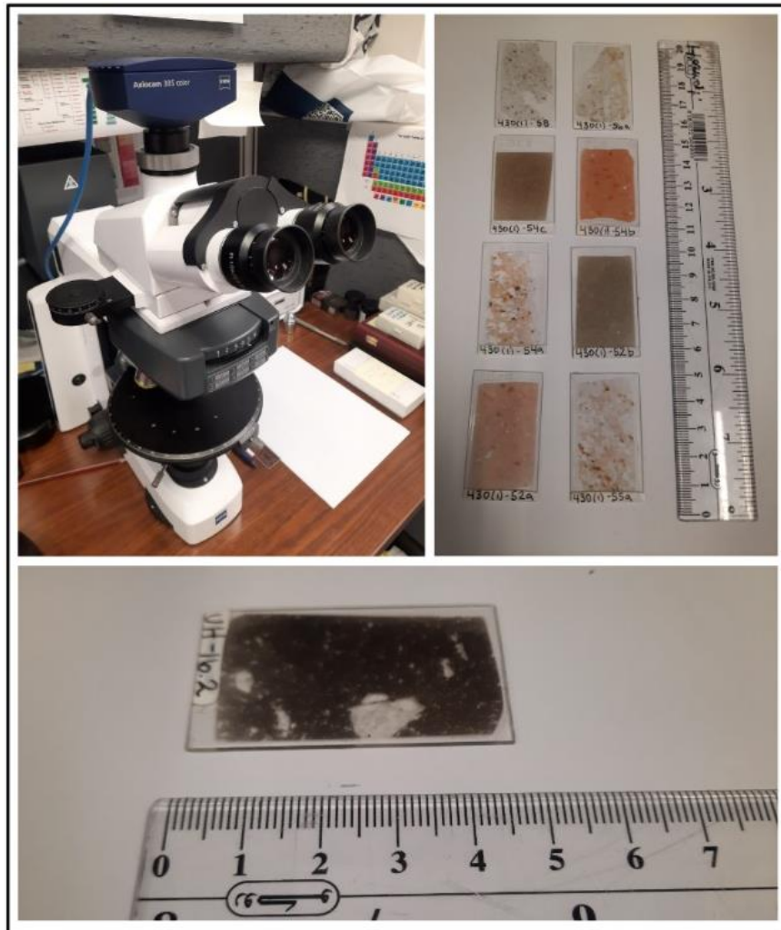
Figure 9 Petrographic microscope and peridotite xenolith thin sections.
