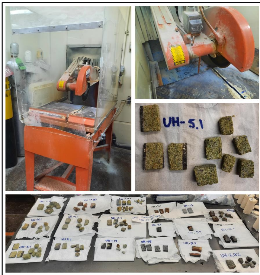
Figure 8 Rock saw machine and prepared peridotite xenolith samples.
