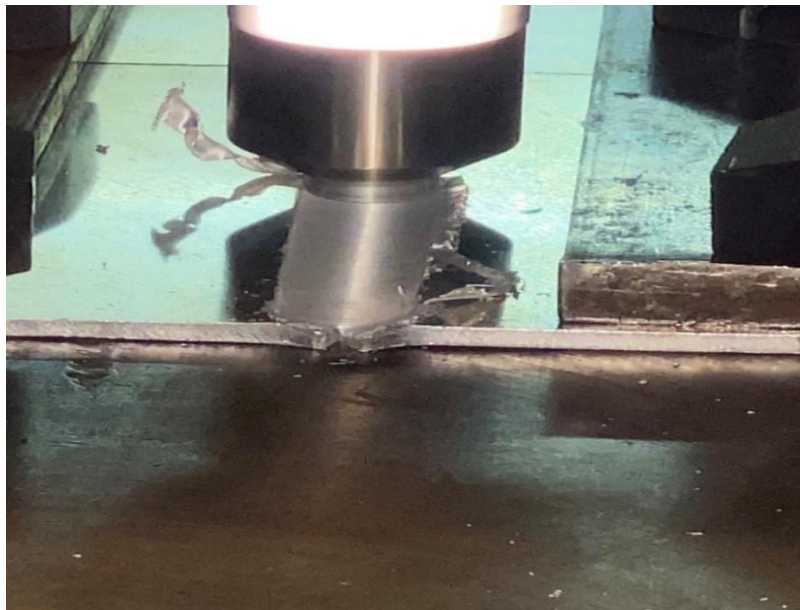
Figure 12: starting of the FSW process.
