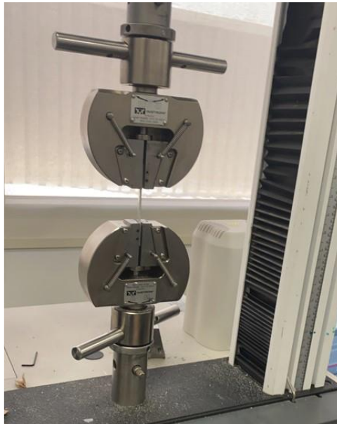
Figure 15: Instron universal tensile test machine
