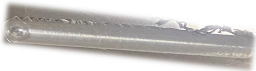
Figure 16a: Surface appearance joint #1
