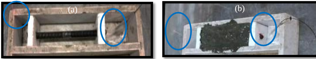
Figure 3. 3: (a) Fiber optic test before concrete casting (b) Fiber optic test after concrete casting
