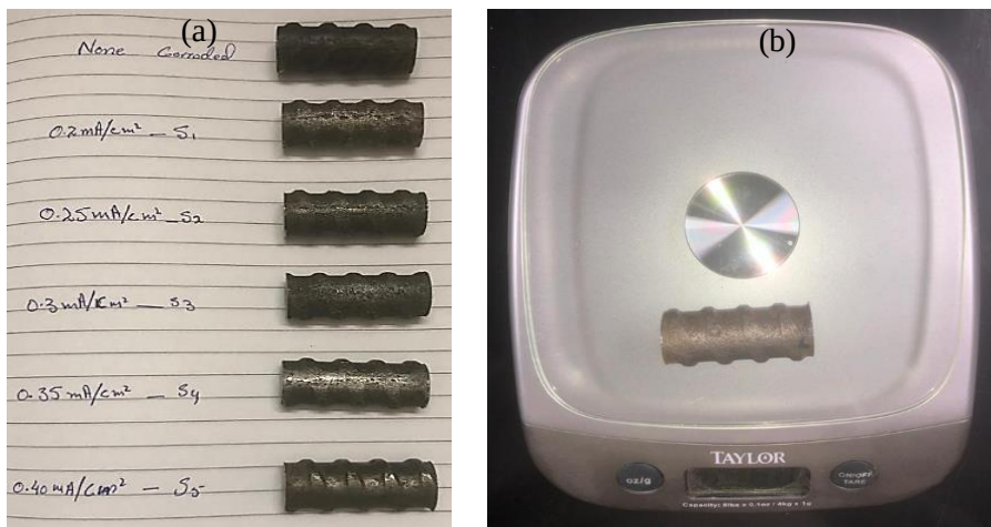
Figure 4. 32: (a) all specimen after cleaning and (b) Weight measurement after corrosion cleaning.
