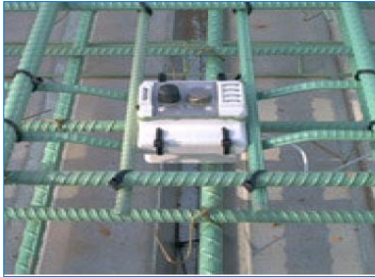
Figure 2. 14: During operation ECI sensor [57]
