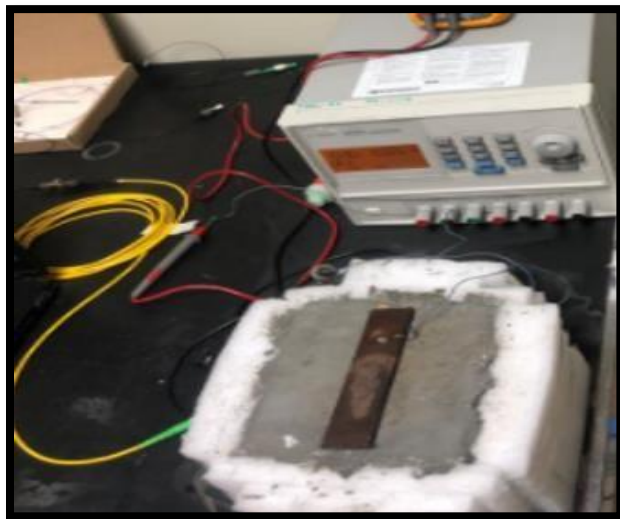
Figure 3. 11: DC current applied on specimen showing counter electrode.
