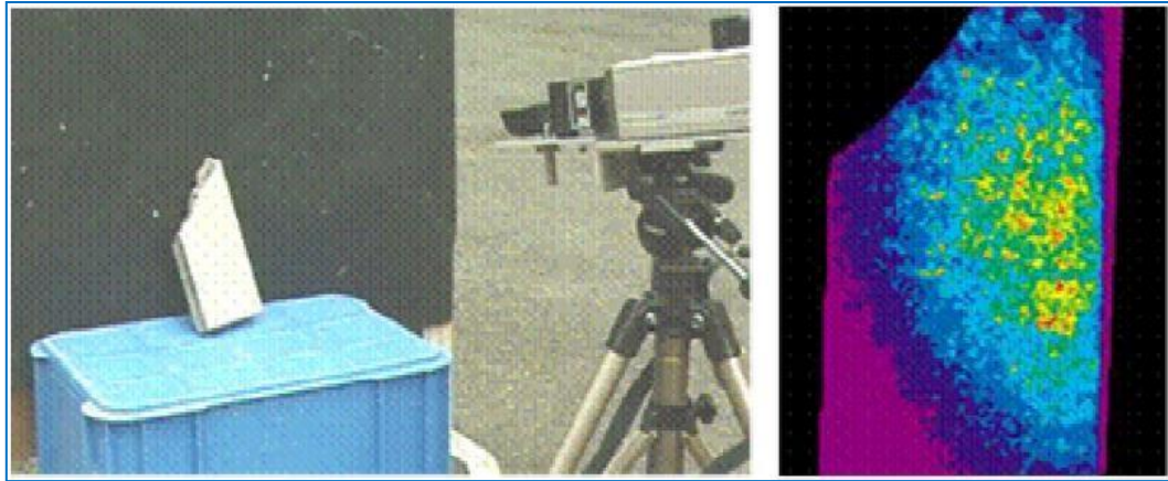
Figure 2. 17: Measurement and result of multi-spectrum camera [106]
