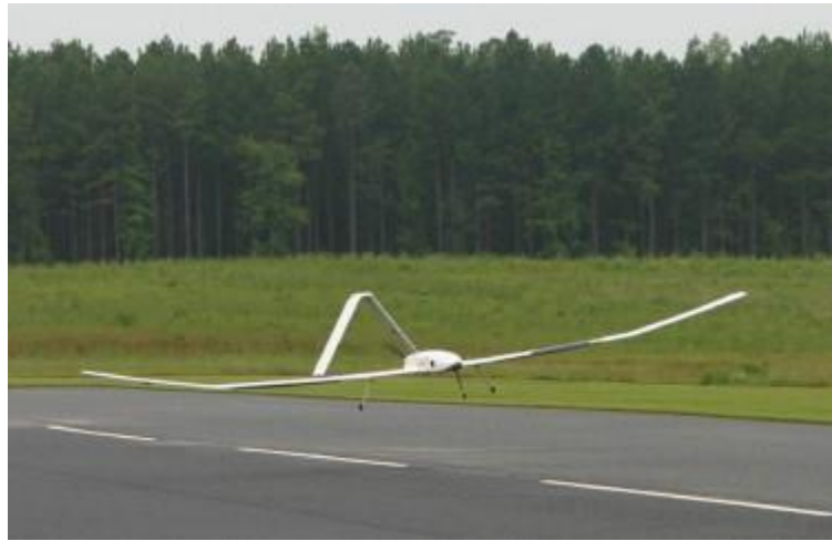
Figure 8. Fuel cell UAV used in the study [14].
