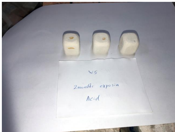
Figure 100 Change in appearance on paste cube after 2-month acid exposure.
