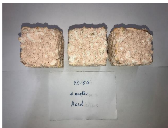
Figure 95 Change in appearance on concrete cube after 4-month acid exposure.
