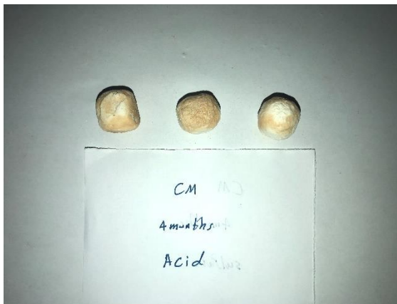
Figure 102 Change in appearance on paste cube after 4-month acid exposure.
