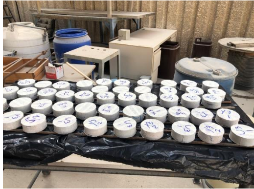
Figure 10 Concrete disk of 50 mm thickness before epoxy coating
