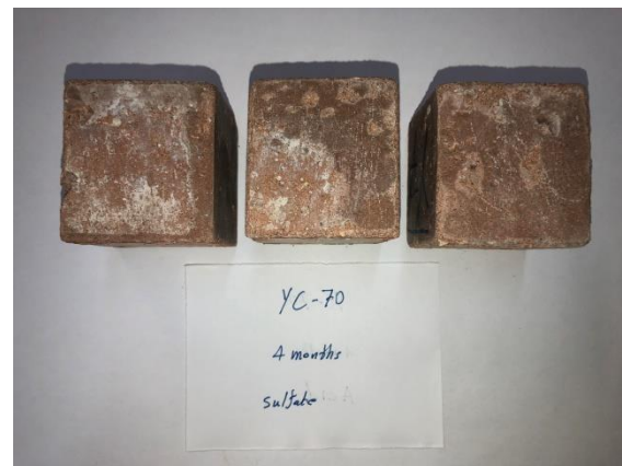
Figure 80 Change in appearance on concrete cube after 4-month sulphate exposure
