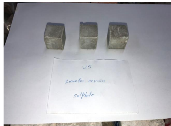
Figure 85 Change in appearance on paste cube after 2-month sulphate exposure.
