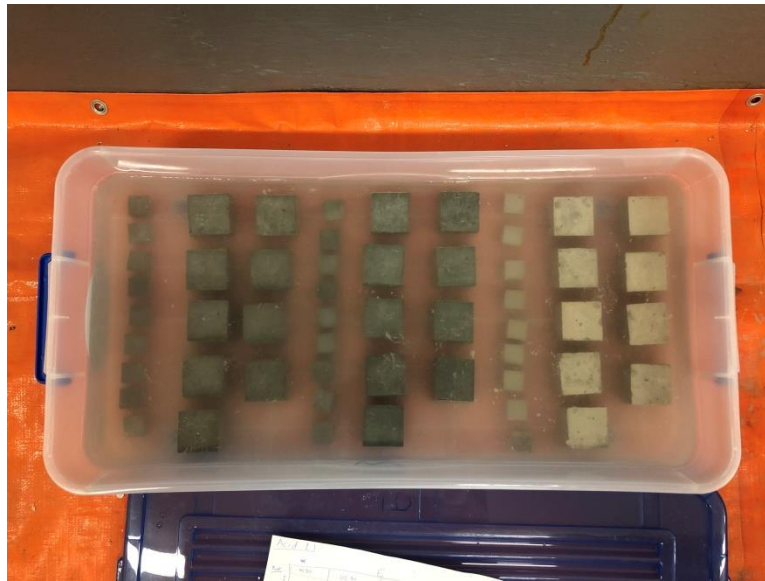
Figure 13 Sulphate and acid samples arrangement in the solution
