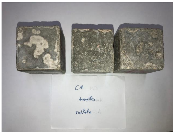
Figure 80 Change in appearance on concrete cube after 4-month sulphate exposure
