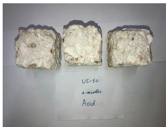
Figure 95 Change in appearance on concrete cube after 4-month acid exposure.
