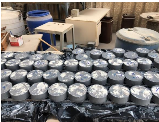
Figure 10 Concrete disk of 50 mm thickness before epoxy coating
