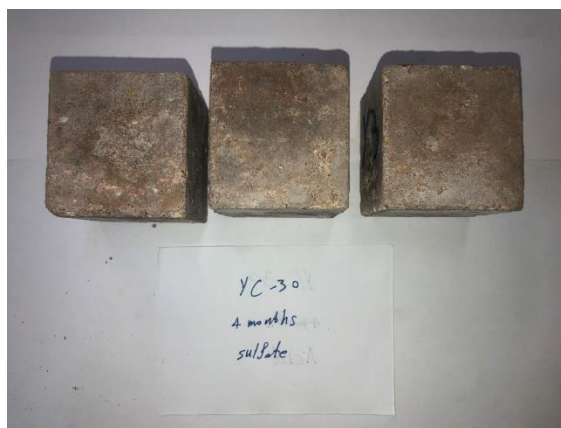
Figure 81 Change in appearance on concrete cube after 4-month sulphate exposure
