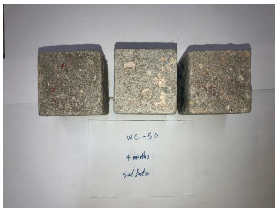
Figure 81 Change in appearance on concrete cube after 4-month sulphate exposure
