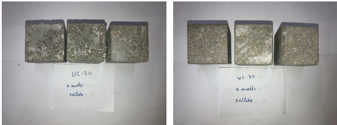
Figure 82 Change in appearance on concrete cube after 4-month sulphate exposure
