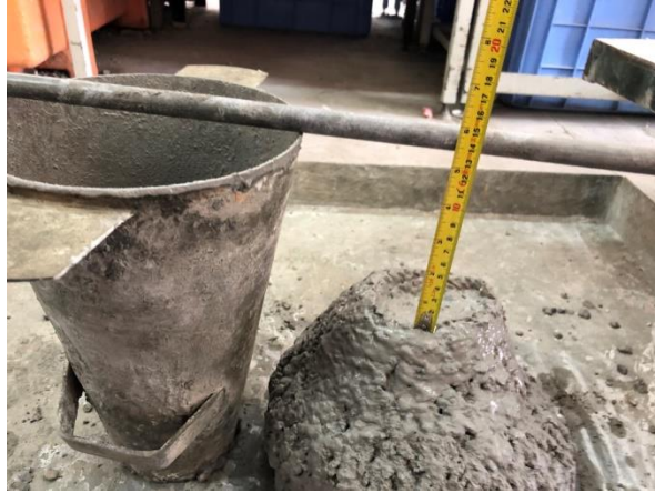
Figure 28: Slump test measuring for UC 70.
