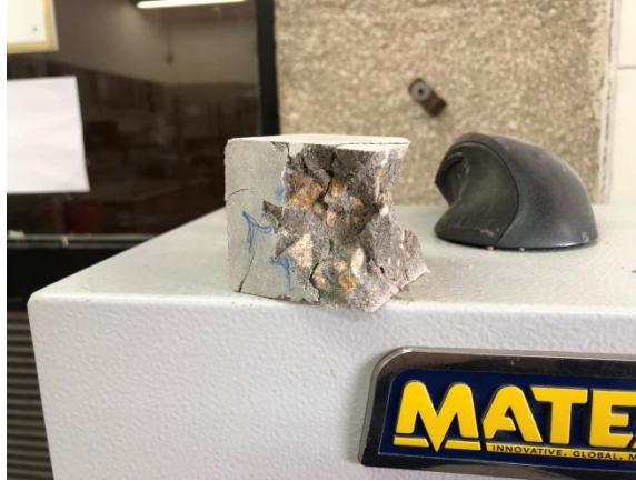
Figure 33 concrete cubic compressive strength cubes after the test
