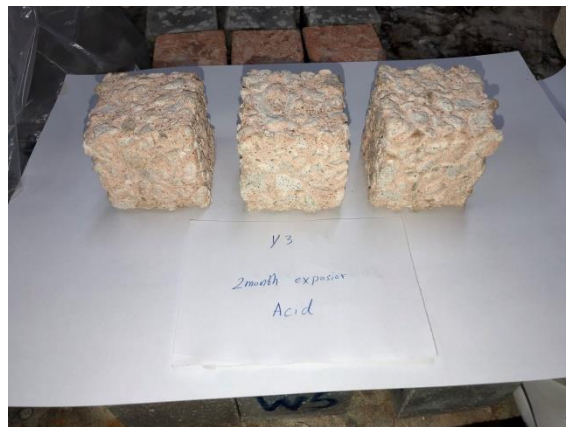
Figure 93 Change in appearance on concrete cube after 2-month acid exposure.
