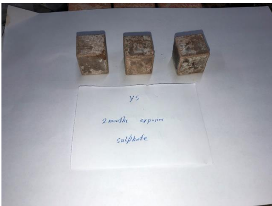
Figure 85 Change in appearance on paste cube after 2-month sulphate exposure.
