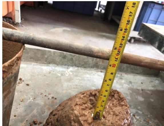
Figure 28: Slump test measuring for UC 70.
