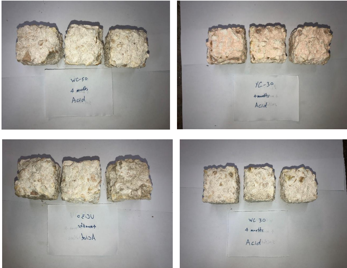
Figure 96 Change in appearance on concrete cube after 4-month acid exposure.
