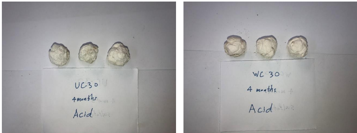
Figure 104 Change in appearance on paste cube after 4-month acid exposure.
