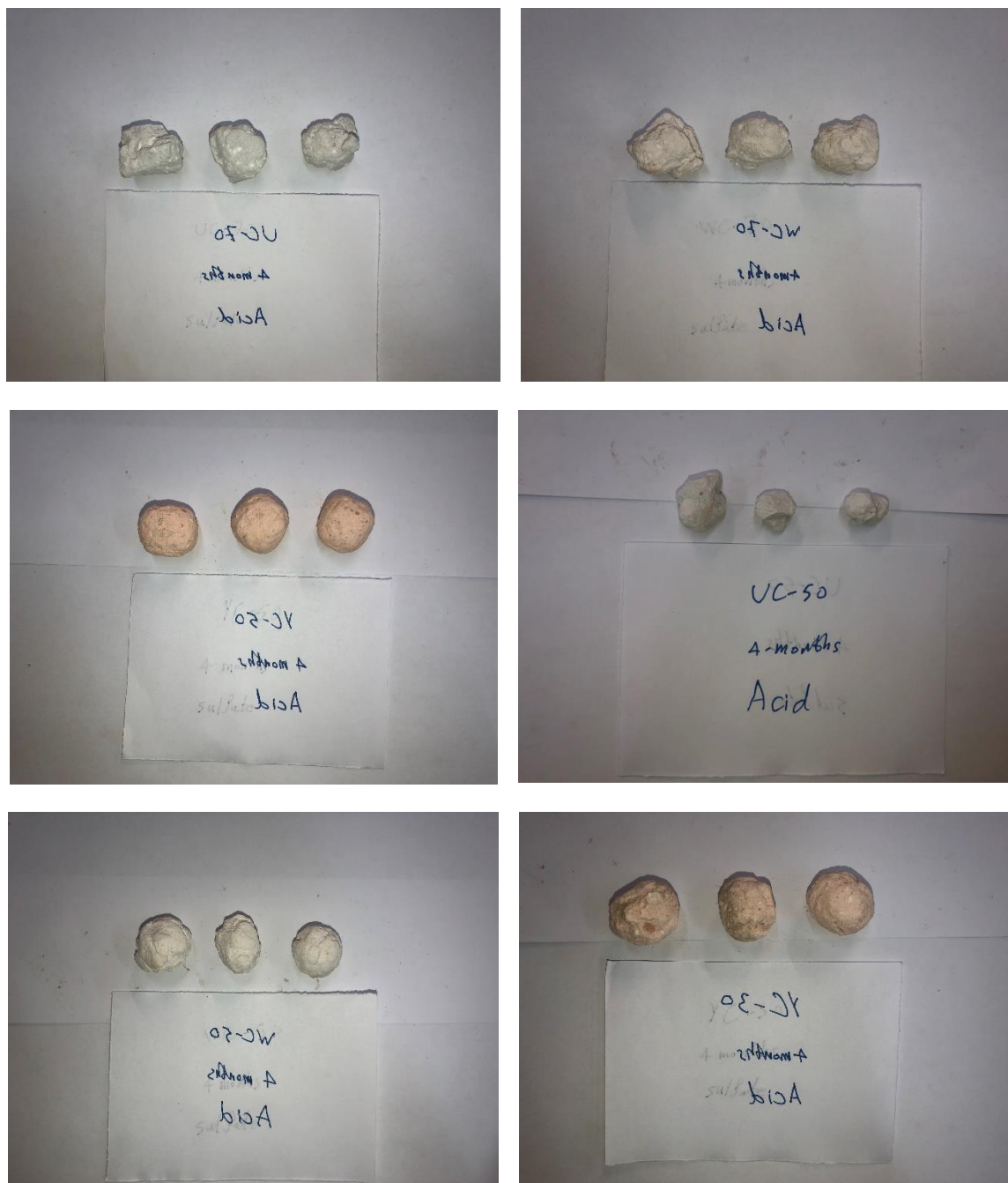
Figure 103 Change in appearance on paste cube after 4-month acid exposure.
