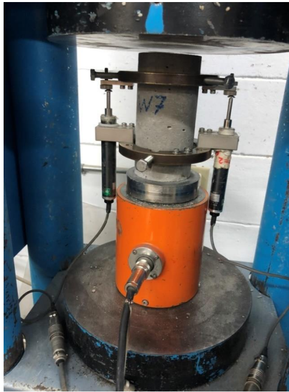
Figure 8 modulus of elasticity measuring setup including load cell, 2LVDTs and holding rings connected to data logger
