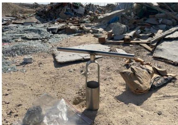
Figure 11 The auger digs a hole to 5 cm depth, and then the sample is collected.
