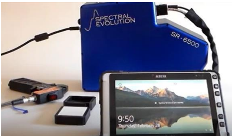
Figure 5 spectroradiometer for in-situ measurements of reflectance
