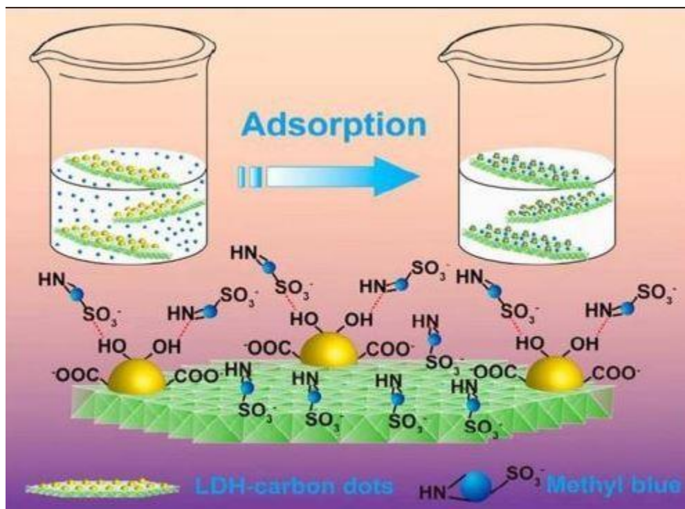
Figure 0-12: Representation of the adsorption of Methyl blue on LDH/C-dot [183].
