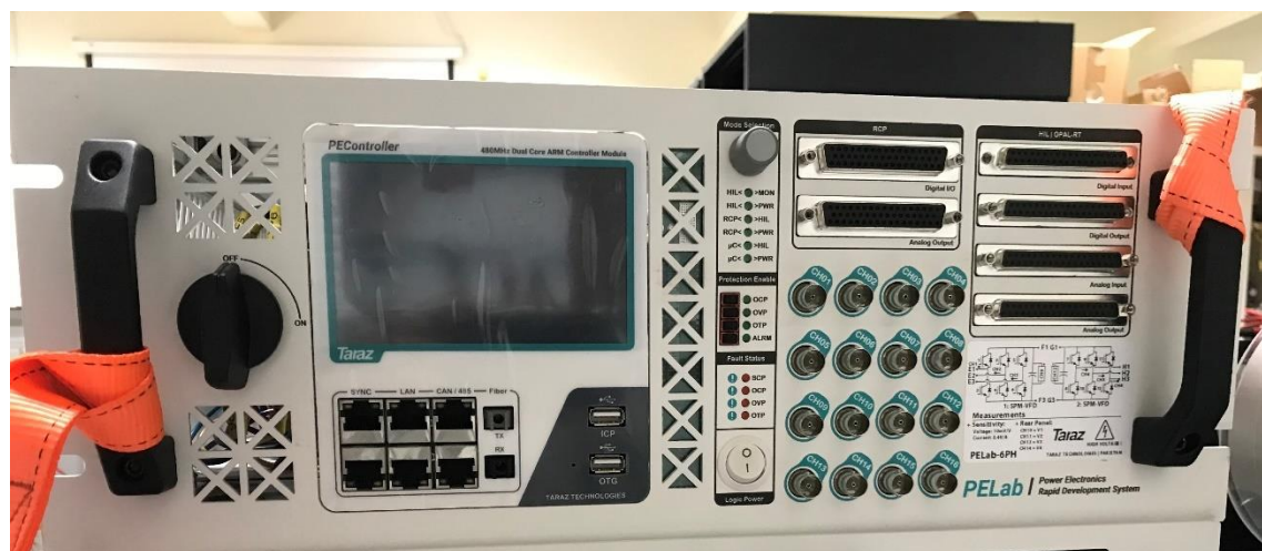
Figure 5.20 PE lab power converters
