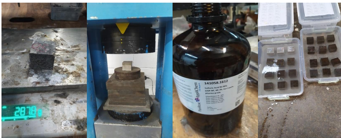
Figure 3-14: Preparation and testing of specimens exposed to acid solution
