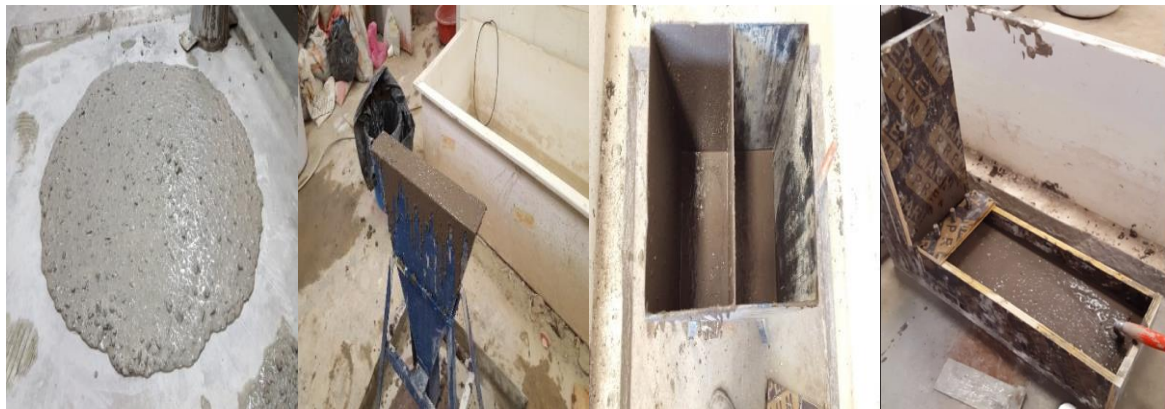
Figure 3-4: Measurement of fresh properties in lab
