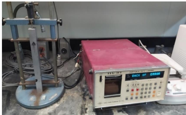
Figure 3-12: Setup used for measuring the expansion of prism specimens
