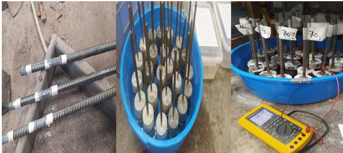
Figure 3-15: Measurement of corrosion potential
