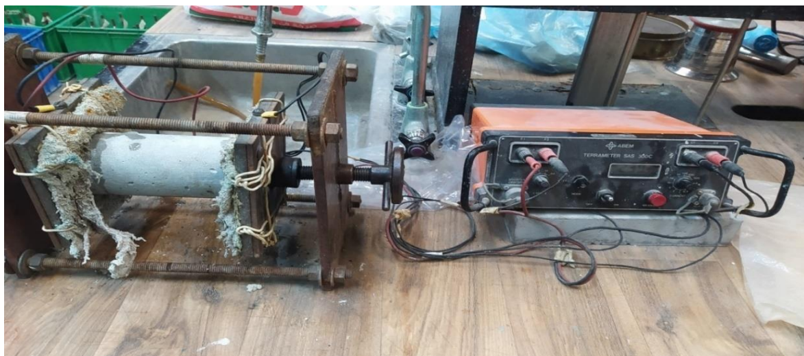
Figure 3-11: Setup for electrical resistivity
