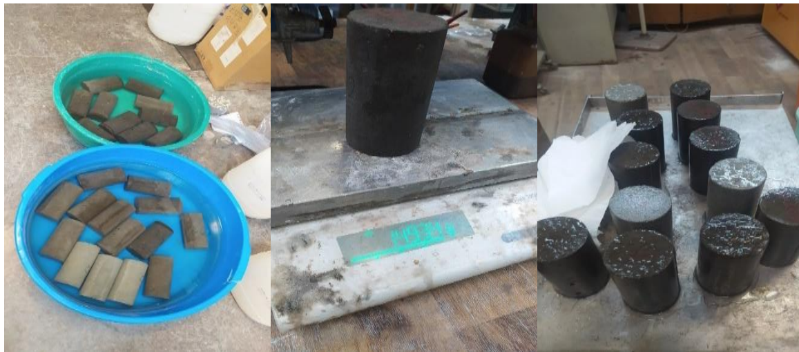
Figure 3-10: Specimens immersed in water for 48 hours
