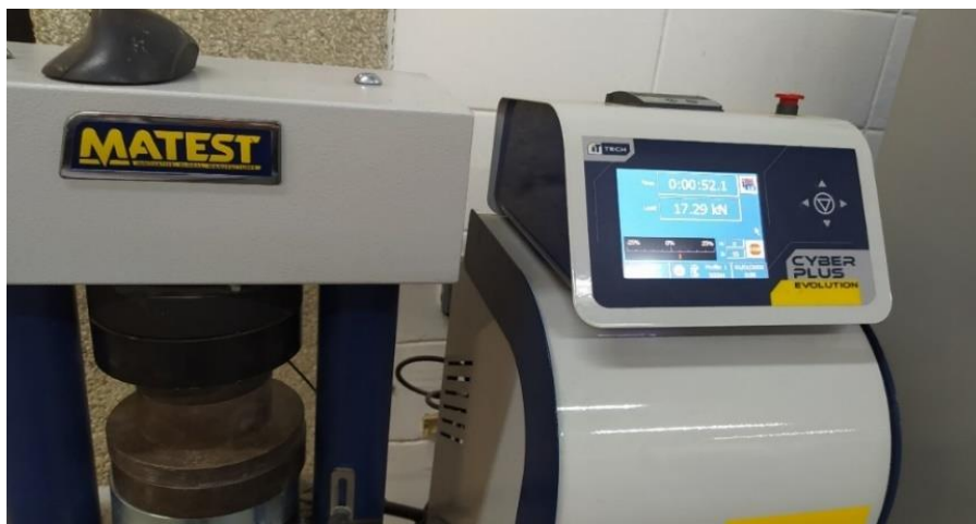
Figure 3-13: Compressive strength machine
