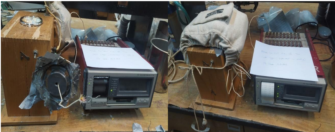
Figure 3-7: Experimental setup used in Heat of hydration
