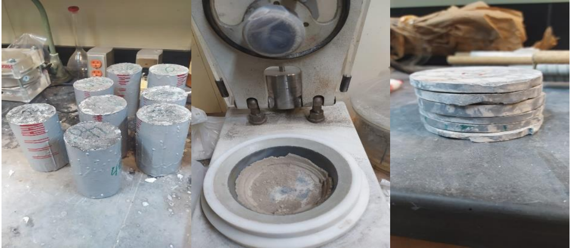
Figure 3-17: Pulverizing of specimens' layers after 3-months of chloride exposure
