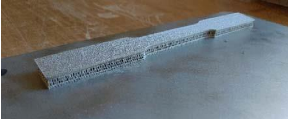
Figure 13: Specimen on the top of the building plate with the support structure [28]
