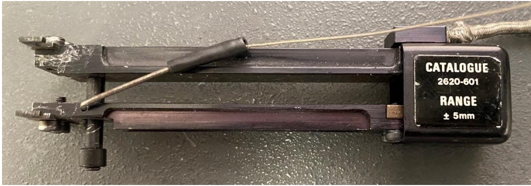
Figure 35: INSTRON CATALOGUE 2620-601 Extensometer
