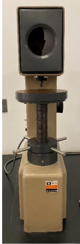
Figure 38: LECO R-600 Hardness Tester Machine (Rockwell B or C)
