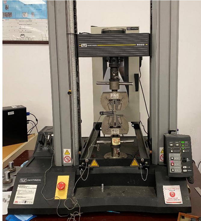
Figure 34: Instron 5569 for Load up to 50kN
