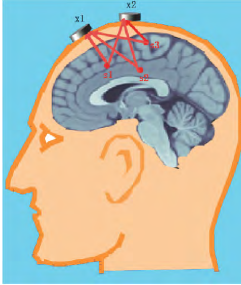
Figure 1.3: Propagation of EEG signals generated from sparse sources through the brain into non-invasive electrodes [3]
