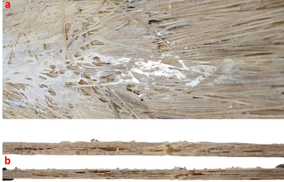
Figure 33: (a) Top view of the large-scale voids, (b) side view of the internal voids between layers
