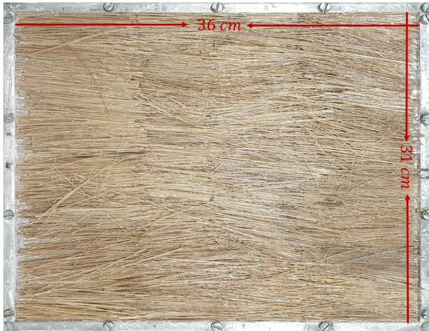
Figure 15: Date palm fibers laid down longitudinally and mixed with the resin in the aluminum mold
