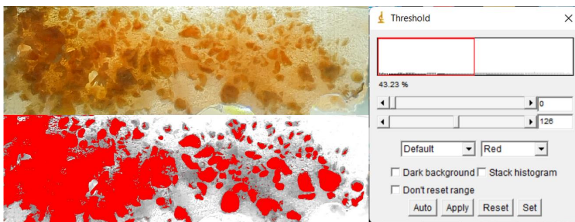
Figure 54: ImageJ analysis of specimen 17wt%-1
