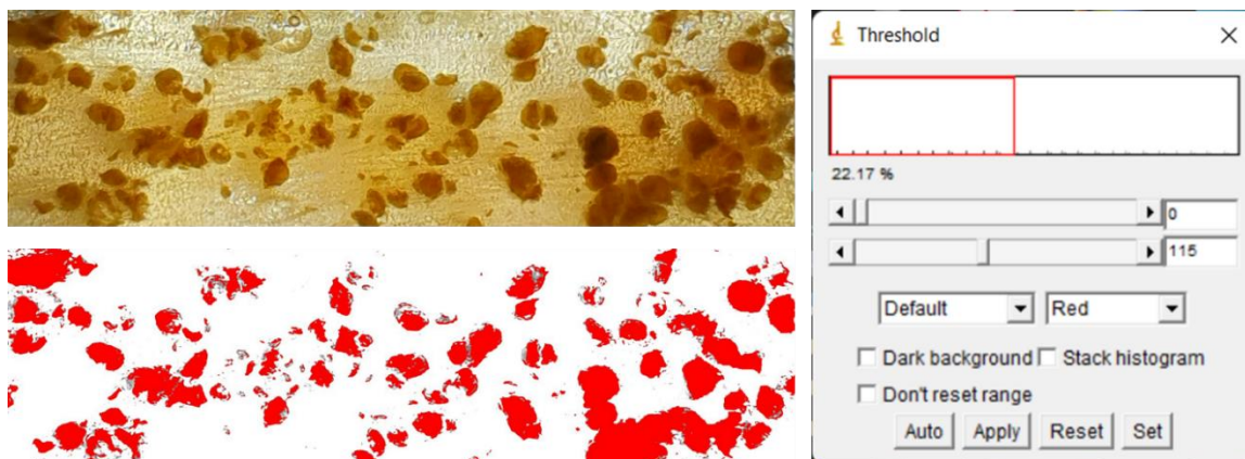
Figure 43: ImageJ analysis of specimen 10wt%-7
