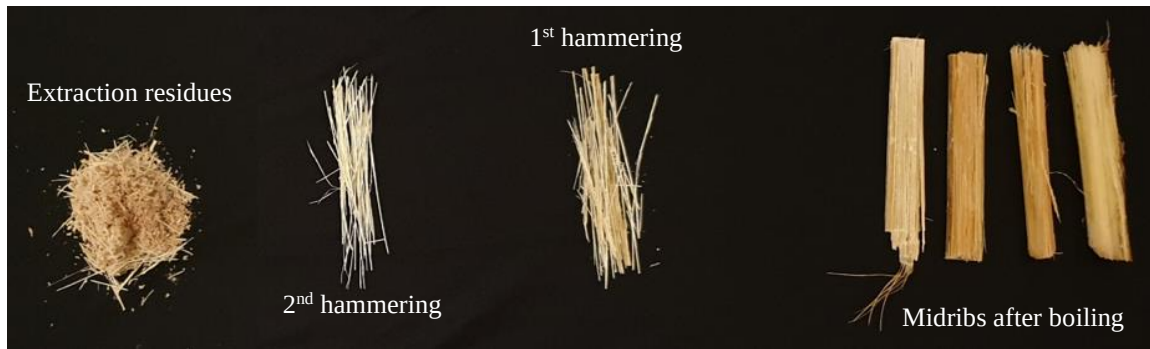
Figure 14: Fibers' extraction levels and the extraction residues
