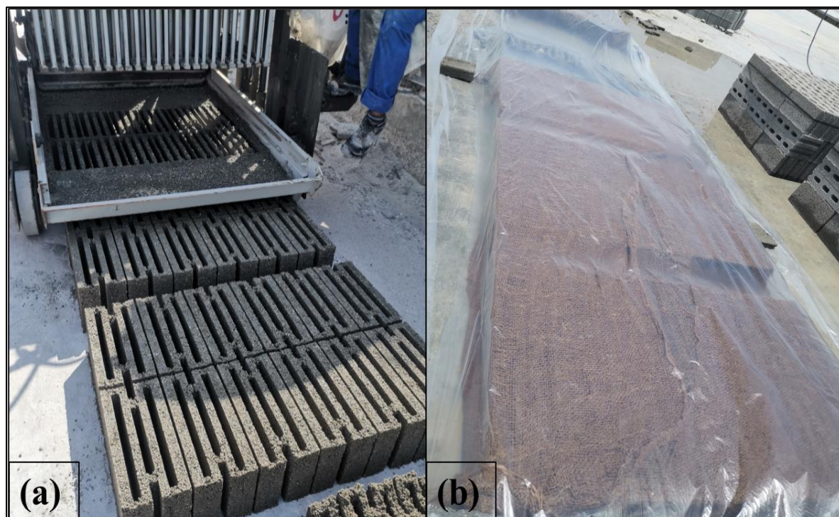
Figure 4: Manufacturing process (a) blocks making machine; (b) blocks covered with burlaps and polyethene sheets
