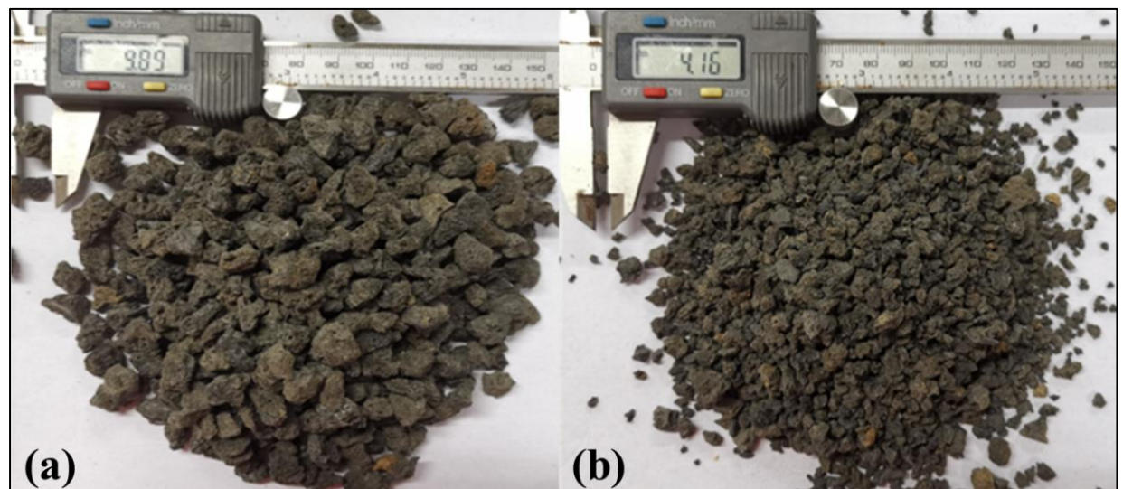
Figure 1: Volcanic Scoria Coarse aggregate (a) VS (# 3/8 in) (9.52mm); (b) VS (# 3/16 in) (4.76mm)
