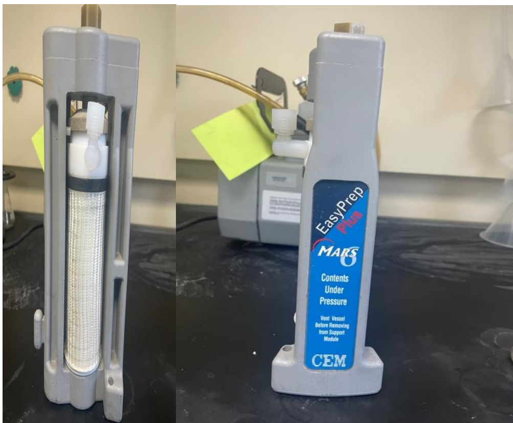
Figure 87 Digestion vessels with pressure and temperature controller
