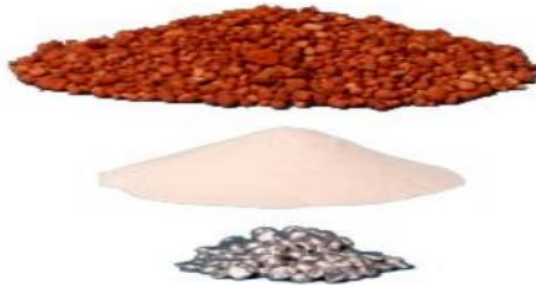
Figure 4 Bauxite from the ore of Aluminum oxide to pure Aluminum
