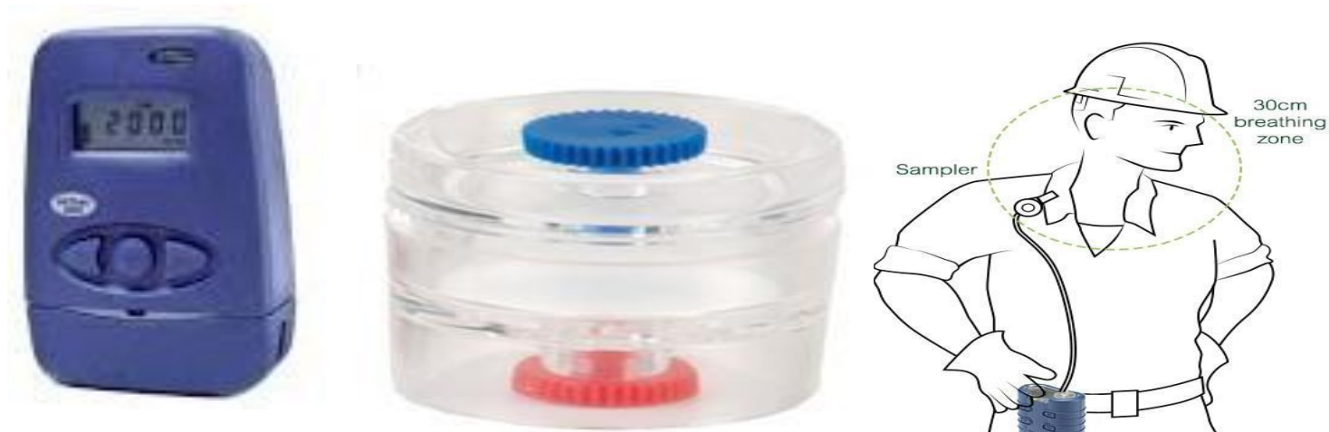
Figure 19 Air Sampling Pump Sampling Media (Cassettes) sampler at Work
