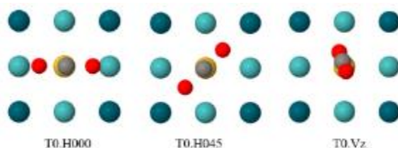
Figure 76. Final locations of CO 2 adsorption on a top-site of Au-atom at PdAu surface (top-view).
