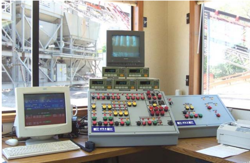
Figure 3 computerized system for batching
