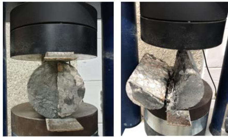
Figure 3.15: Split tensile test between UHPC and normal concrete
