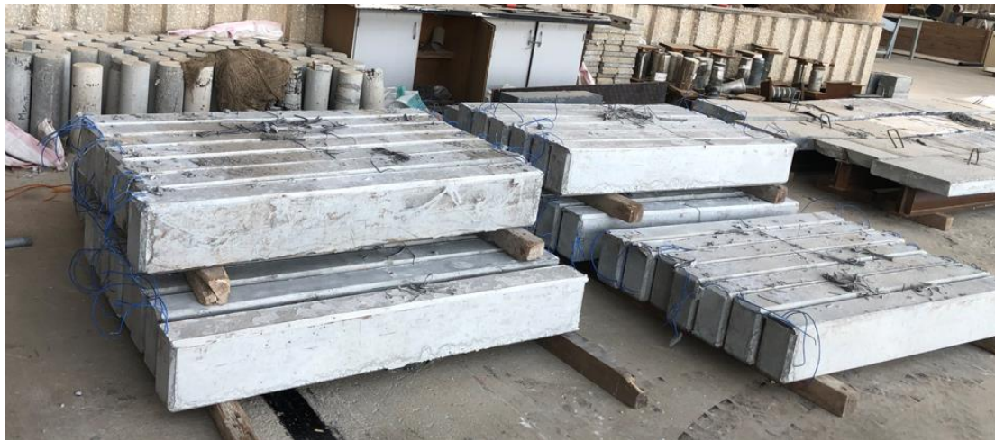
Figure 3.7: RC beam specimens laid inside the KFUPM structural lab
