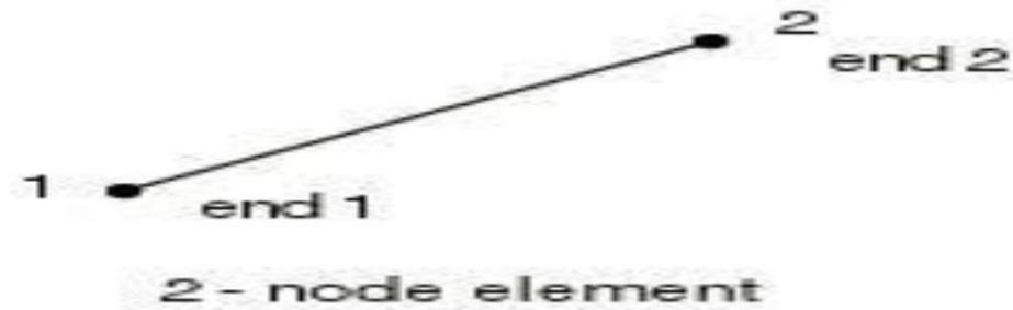
Figure 6.7: A 2-D noded linear 3-D truss element
