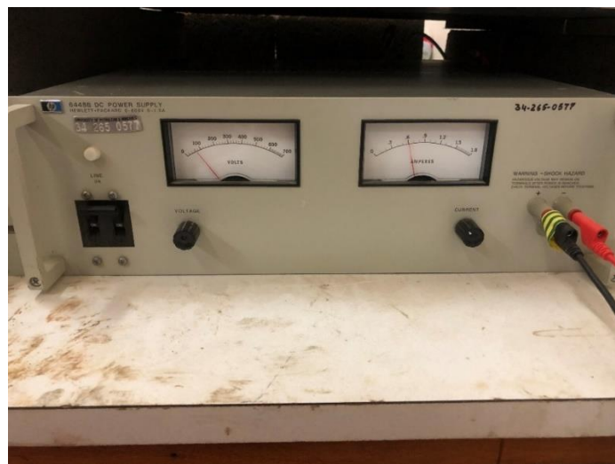
Figure 3.17: DC power source used to induce current to RC beams.
