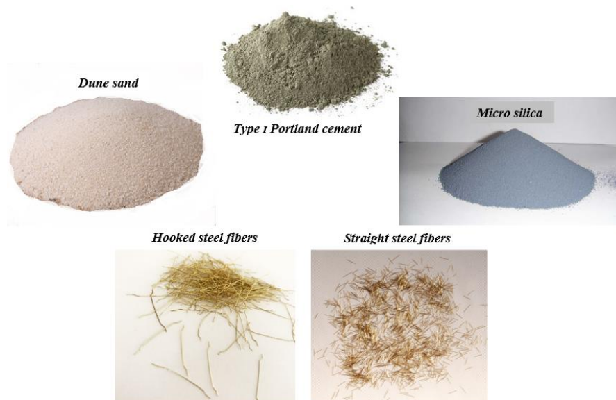
Figure 3.11: UHPC ingredients used for strengthening.
