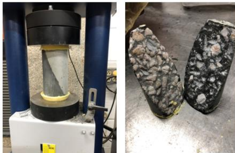
Figure 3.16: Slant shear test between UHPC and CFRP
