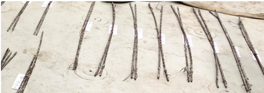
Figure 3.31: Set of corroded bars after being extracted from the beam specimens.
