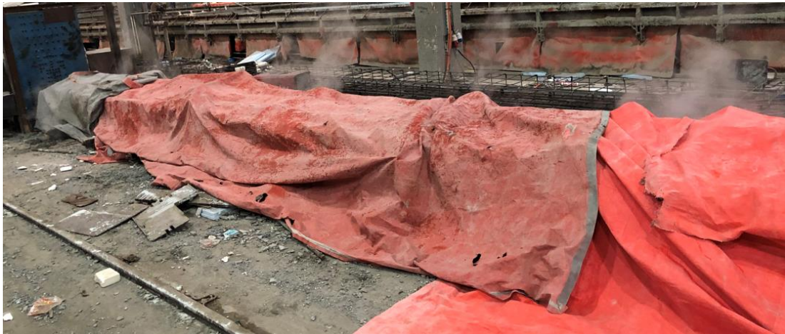
Figure 3.6: Steam curing of concrete beam specimens at PRAINSA factory
