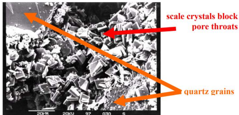
Figure 31 – Formation damage due to scale deposition
