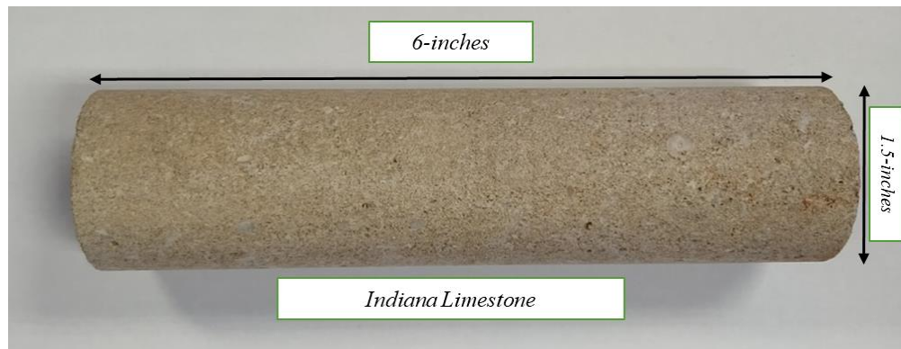
Figure 18 – Indiana limestone rock sample with its dimensions
