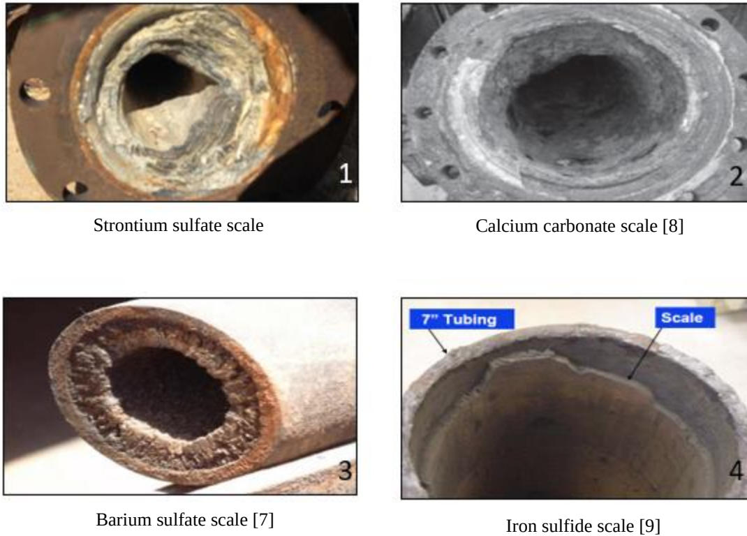
Figure 1 – Precipitation of different inorganic oilfield scales in the production tubing
