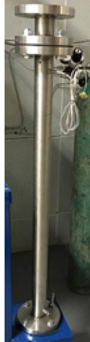
Figure 3.1: Schematic representation (left) and experimental setup (right) of swirl-stabilized model gas turbine combustor.
