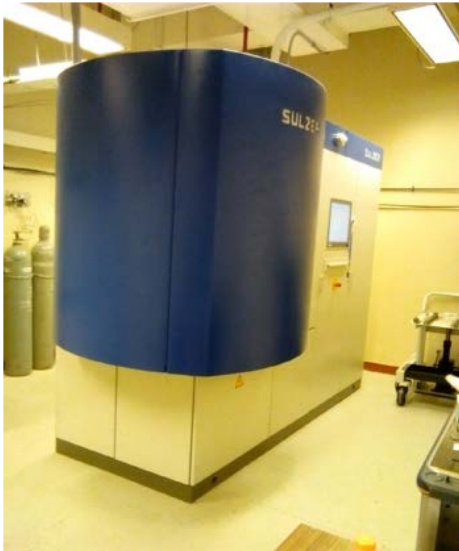
Figure 3.2: Cathodic arc deposition PVD Equipment [5]
