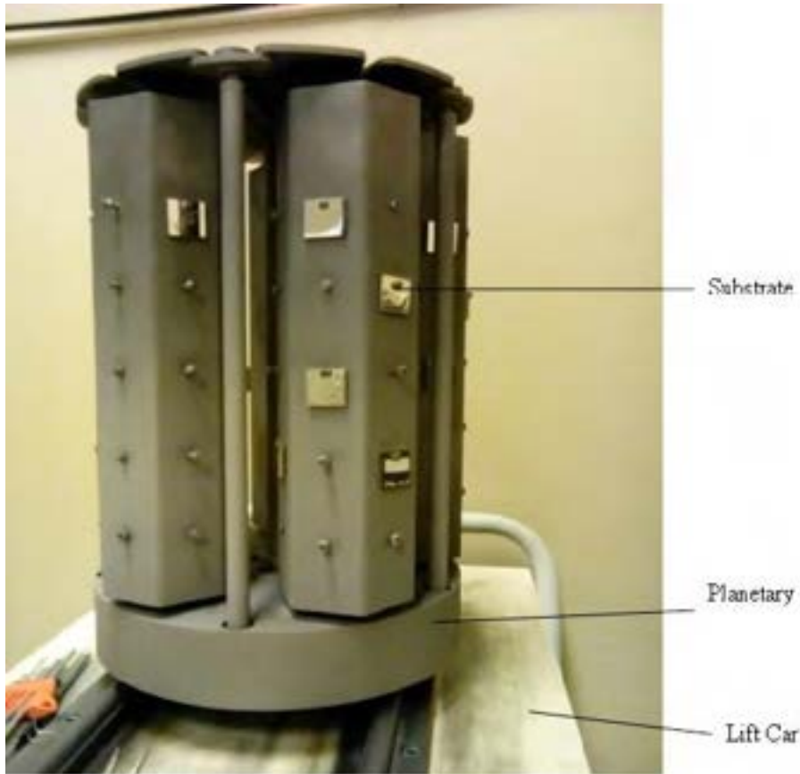
Figure 3.3: Fixture with substrates attached for planetary rotation [5]
