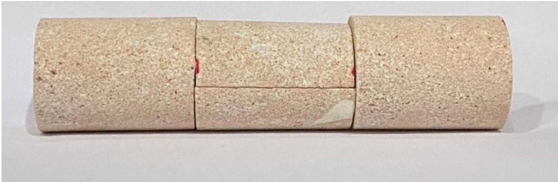
Figure 10: Pink desert limestone composite core
