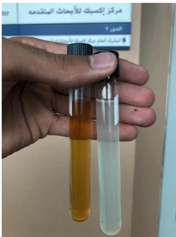
Figure 23: Broken fluid at 300^{\circ}\text{F} on the left and prepared fluid before testing under HPHT on the right
