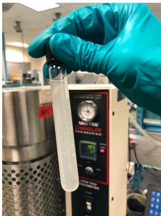
Figure 11: Prepared mixed fluid - 10 wt. % GLDA, 50 pptg CMHPG, PW.
