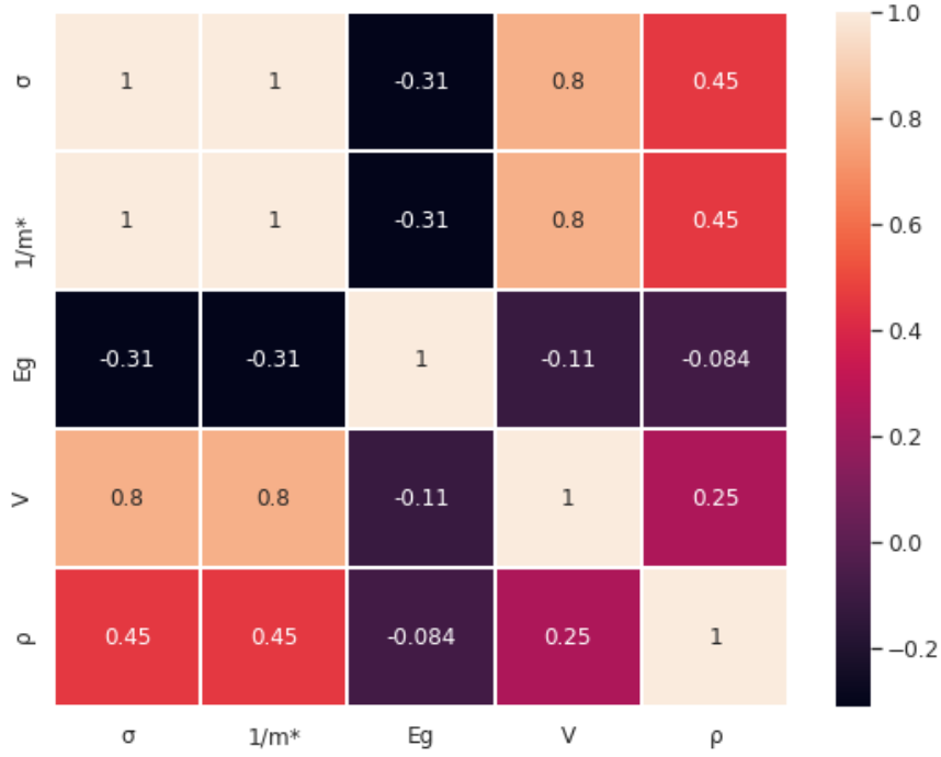
Fig 4-3 Correlation matrix for electrical conductivity and the considered physical features.
