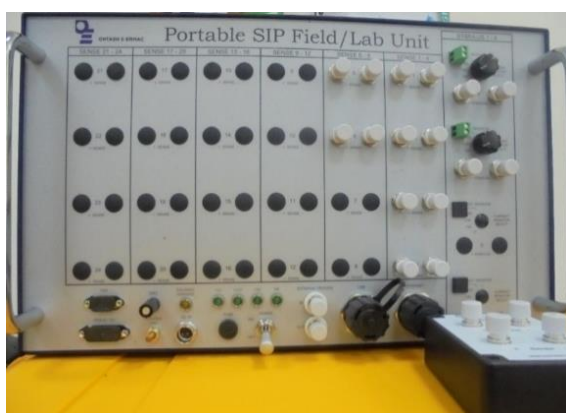
Figure 5 Portable Field/Lab Spectral Induced Polarization (PSIP) instrument
