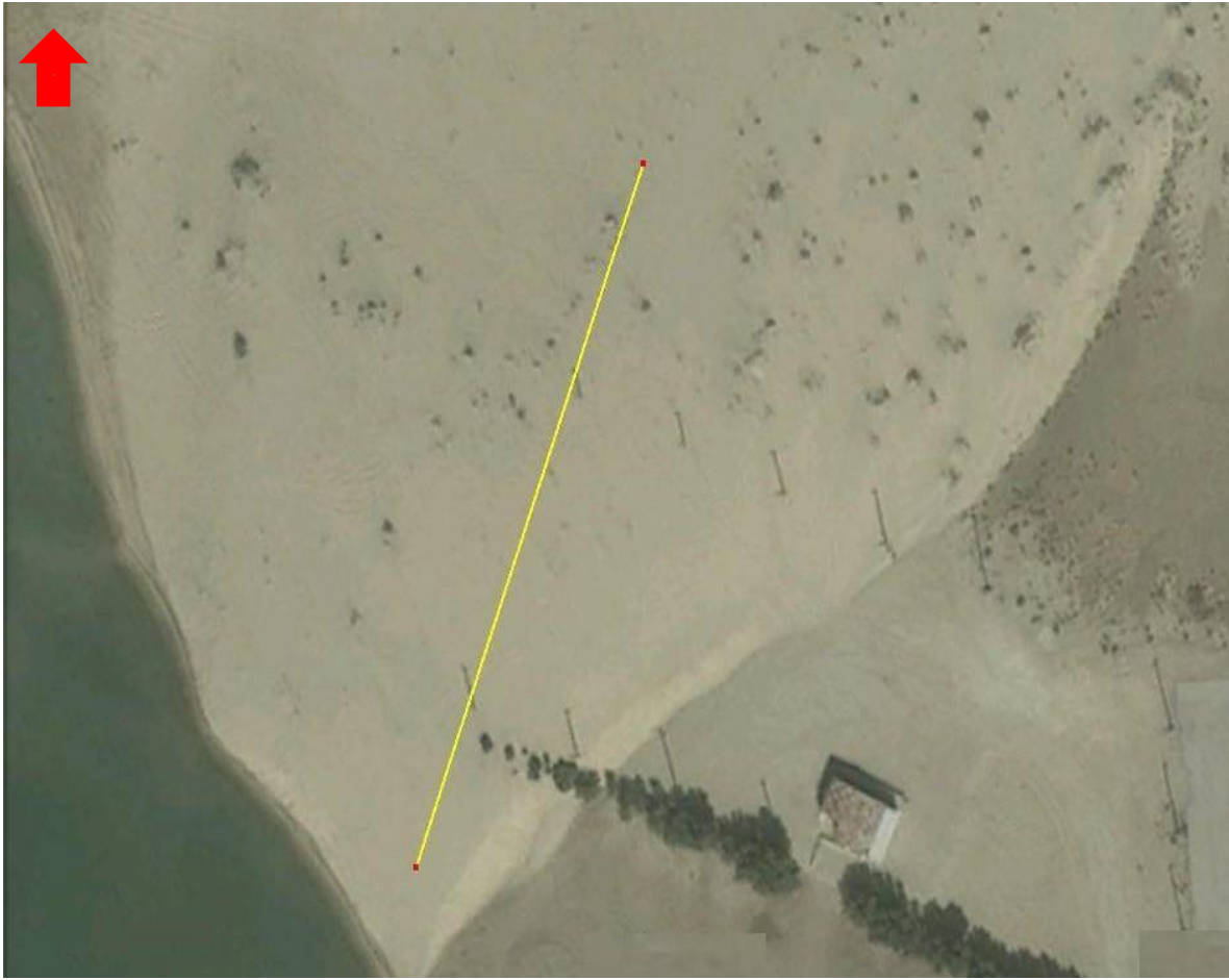
Figure 15. Seismic line location over the sand dune at KFUPM Beach
