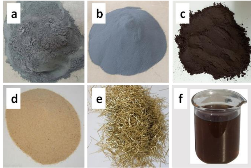
Figure 3.1: a) OPC, b) SF, c) HP, d) Dune sand, e) Steel fibers, f) Superplasticizer
