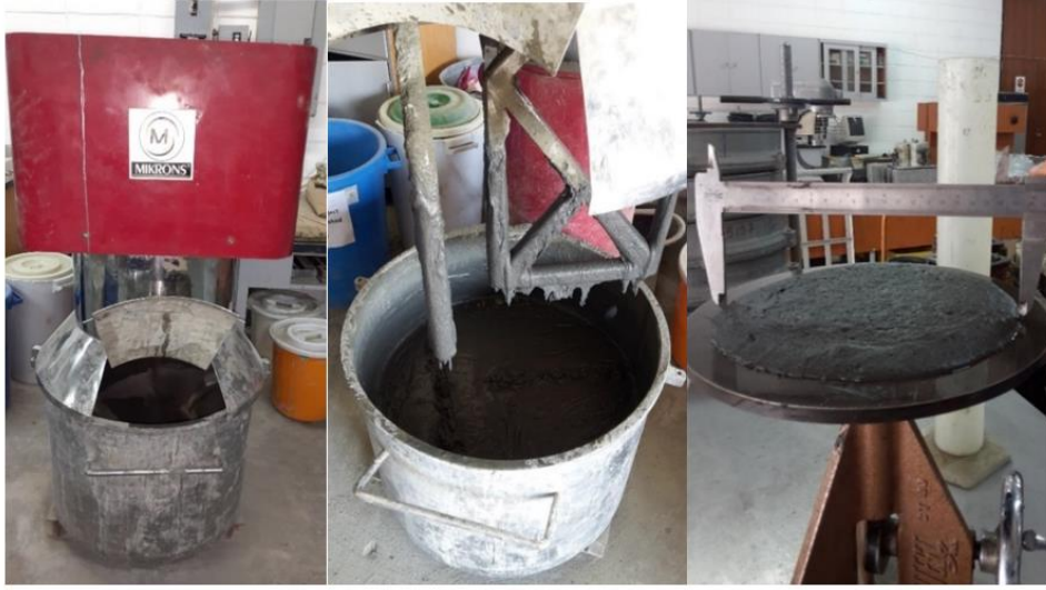
Figure 3.2: Planetary mixer (left), UHPC mixture (center), flow table test (right)
