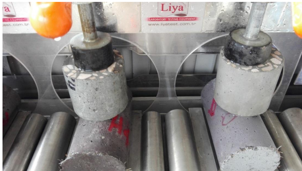
Figure 3.4: Mechanical grinder for smoothening the concrete casting surface
