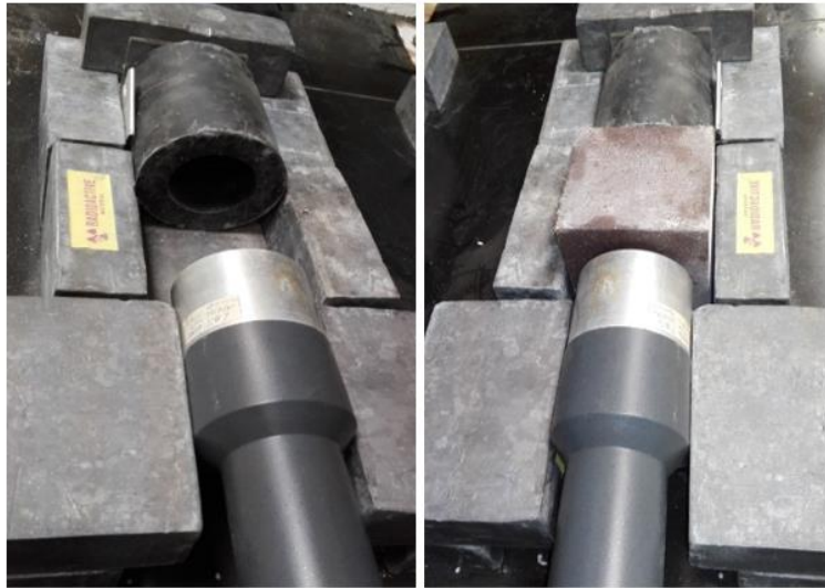
Figure 3.15: Gamma radiation shielding test, with and without specimen
