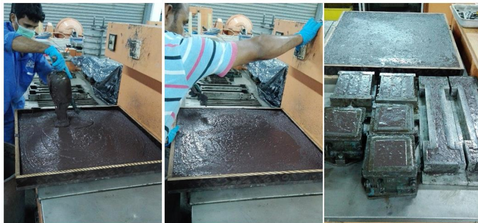
Figure 3.3: Concrete pouring into the moulds
