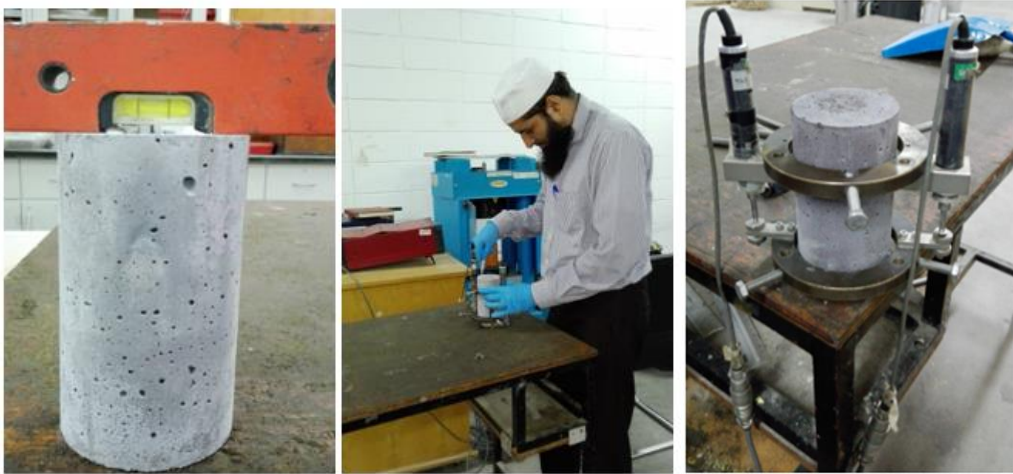
Figure 3.5: Testing setup for compressive strength and modulus of elasticity tests
