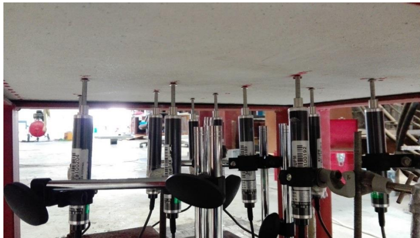
Figure 3.13: LVDT's under the slab for measurement of deflections
