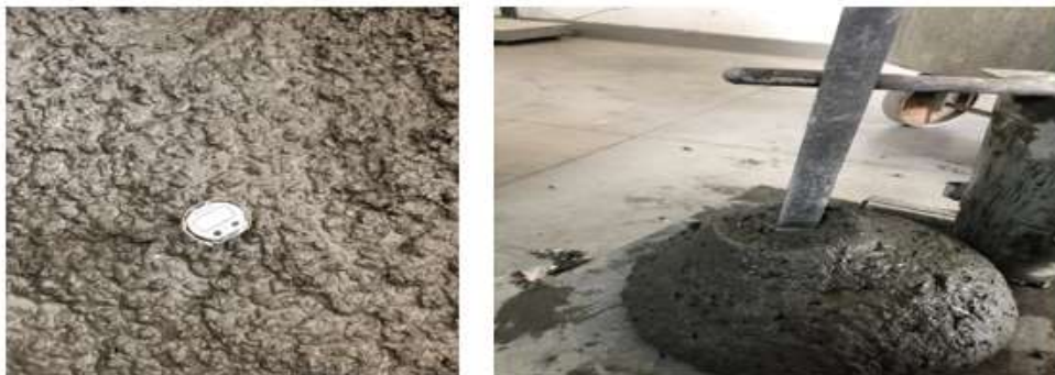
(c) Measuring the temperature and slump of the SC
