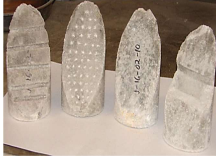
Figure 2.6 Slant shear test specimens with different substrate surface preparation; grooved, chipped, smooth, and shear key [19]
