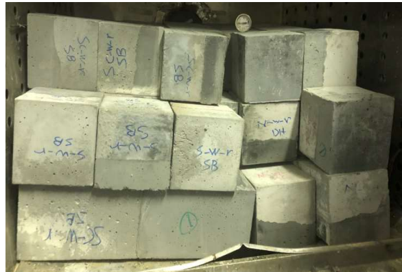
Figure 3.6 Process of wet-dry and heat-cool cycling exposures
