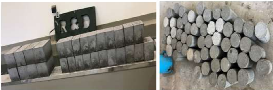
(f) De-molding of the specimens
