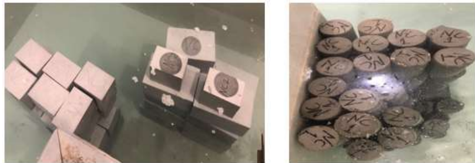
(g) Water curing of the concrete substrates (28 days)
