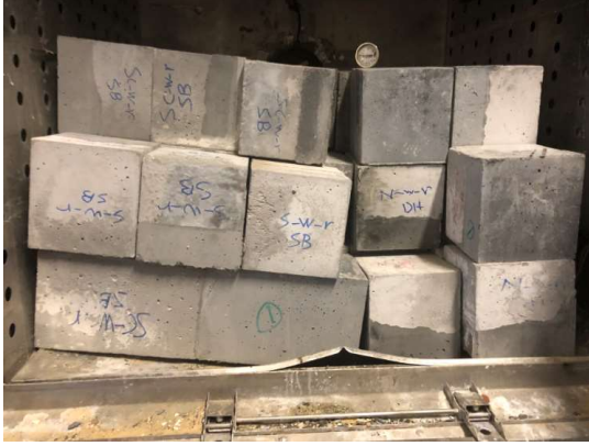
(f) Heat curing condition (12-hour at 60 °C)
