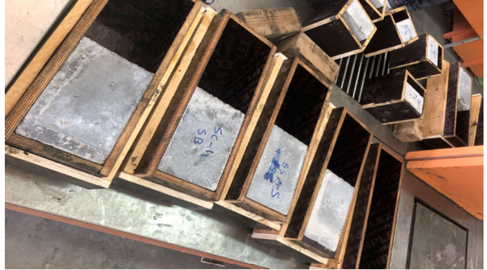
(b) Substrate positioned inside the mold before casting the overlay
