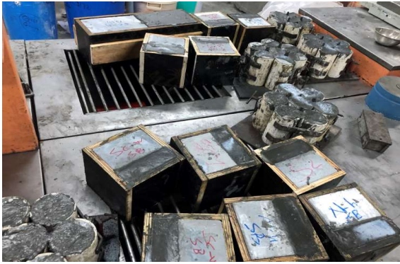
(c) Casting of UHPC
