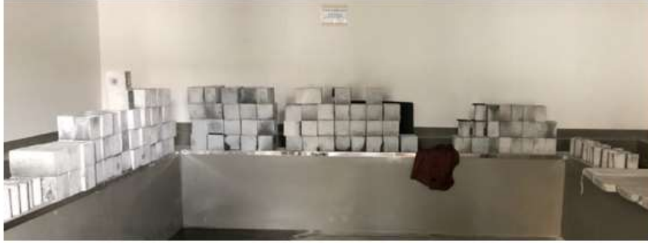
(h) Specimens were then put at room temperature 22 \pm 2 °C and relative humidity of 56% up to 3 months
