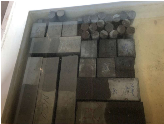
Figure 3.6 Process of wet-dry and heat-cool cycling exposures
