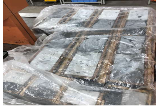
(d) Covering of test specimens with plastic sheets
