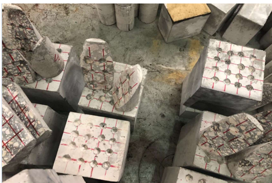
Figure 3.3 Drill holes preparation; evenly spaced at 30 mm c/c distance and 5 \pm 2 mm depth of the hole, and sandblast roughness; at 2 mm an average depth
