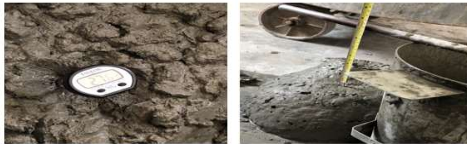
(b) Measuring the temperature and slump of the NC
