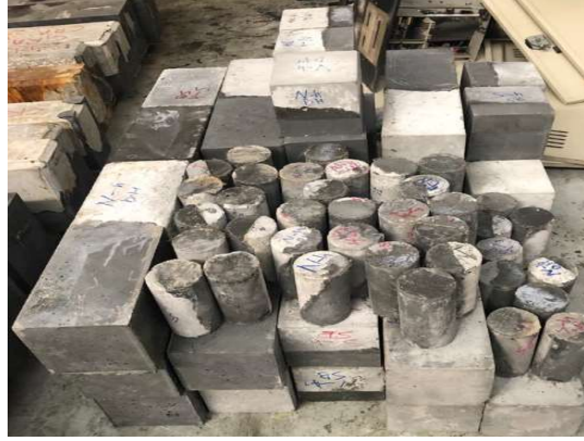
(g) The composites left to dry before testing
