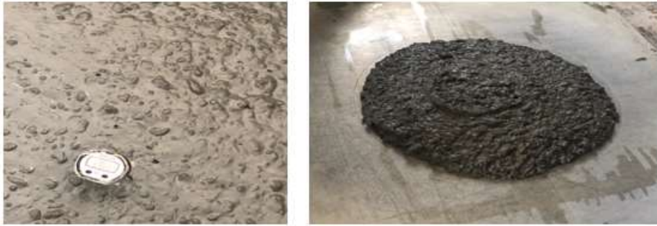
(d) Measuring the temperature and slump of the SCC
