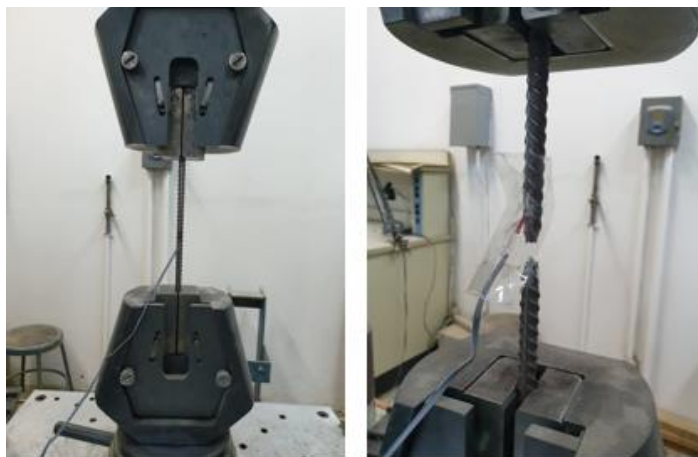
Figure 23: Steel tensile test
