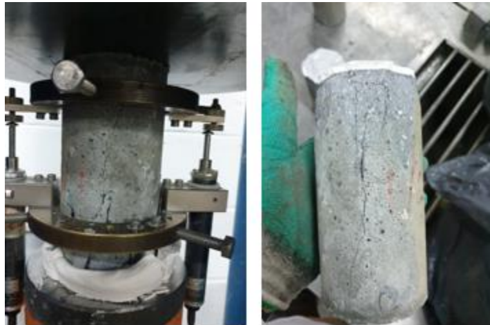
Figure 28: Modulus of elasticity test for the repair material MasterFlow 980 .
