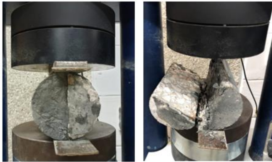
Figure 29: Split tensile test between UHPC and normal concrete
