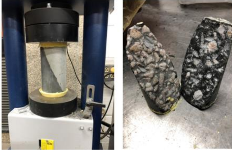
Figure 30: Slant shear test between UHPC and CFRP
