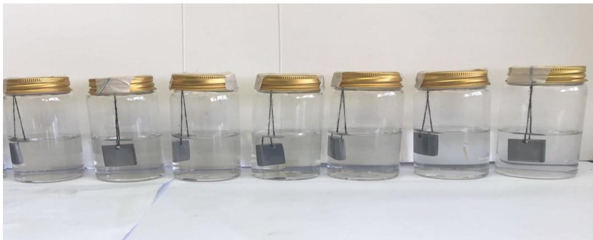
Figure 27: wt loss exp. at different concentrations
