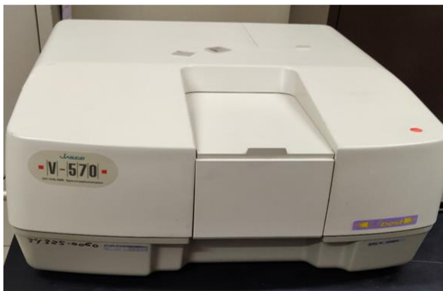
Figure 2.12 The JASCO V-570 double beam spectrophotometer.
