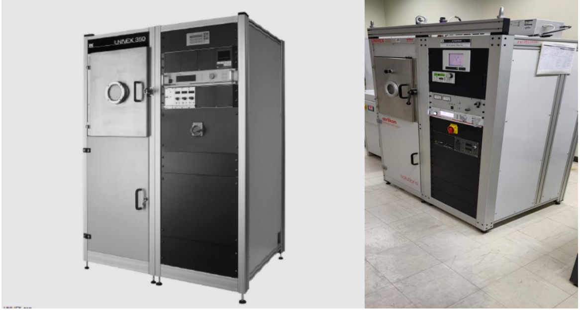
Figure 2.2 Oerlikon Univex 350 system that was used for the deposition of the films.
