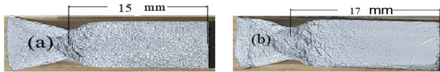
Figure 5-5: SDSS SAF 2507 fracture surface of CT specimens, (a) BM and (b) FSPed.
