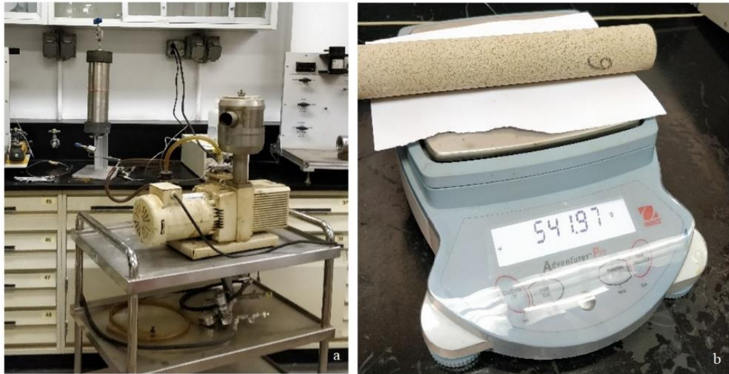
Figure 6. 3 Vacuum pump and core holder for water saturation process, b) balance for measuring the core mass
