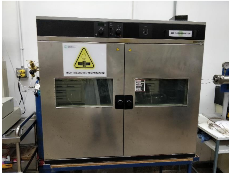
Figure 6. 7 Oven for steam generation
