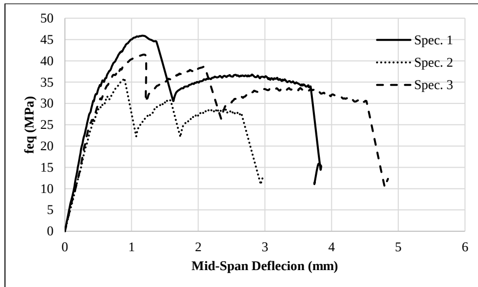
Figure B10: Stress/deflection of mixture U100H water cured
