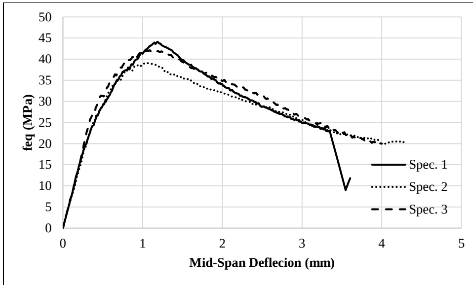
Figure B7: Stress/deflection of mixture U70H steam cured
