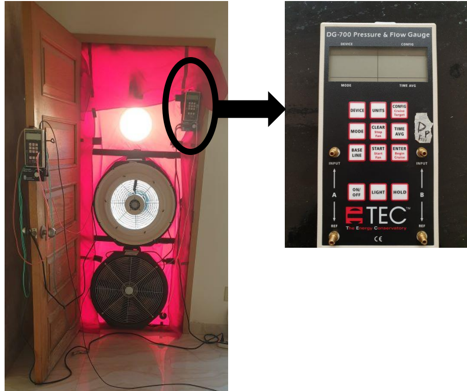
Figure 3.3: Used blower door assembly and pressure gauges
