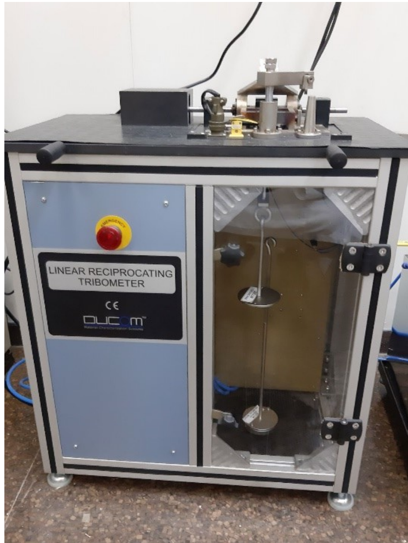
Figure 3- 7 Linear reciprocating tribometer
