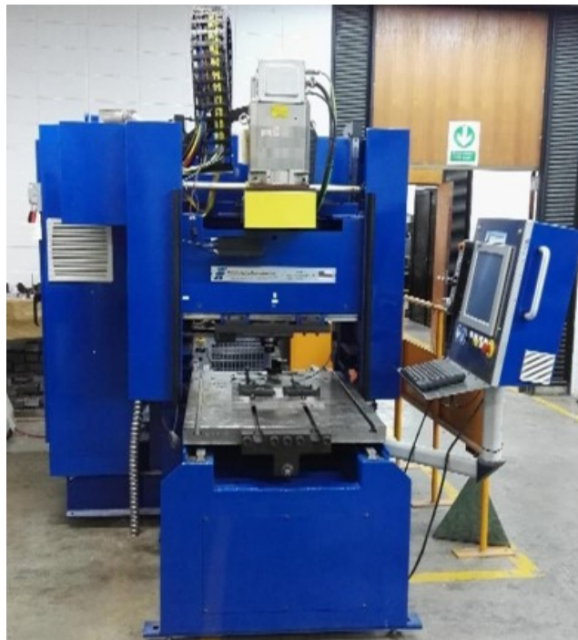
Figure 3- 1 RM-1 FSW machine
